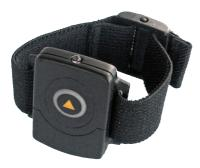
The LaserScope comes with a Remote Transmitter to make ranging more convenient. Position the Remote Transmitter on the fore end of a rifle as shown below. It can also be positioned on the Objective Bell of the LaserScope. The LaserScope is Remote-capable for a full 2 hours every time the Main Switch is depressed.
