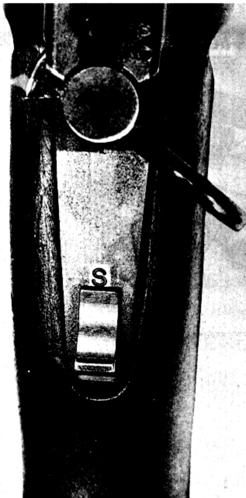
Figure 9-3. Location of the safety in the safe position.
