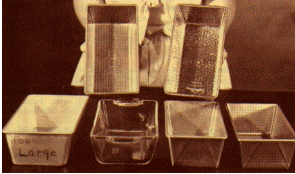
Dull Pan Upper Left Has Been Tempered. Shining Pan Upper Right Has Not
