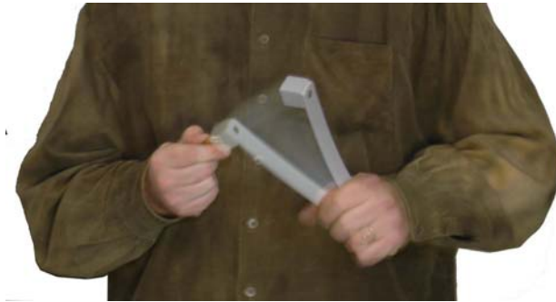
The bumping of a lock using the 'Tomahawk'.
