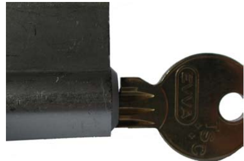
A picture showing the gap between the lock and the shoulder of a 'minimal movement' bump key.
