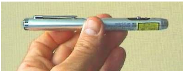
Inexpensive laser pointer (1 mw, 650 nm red)
