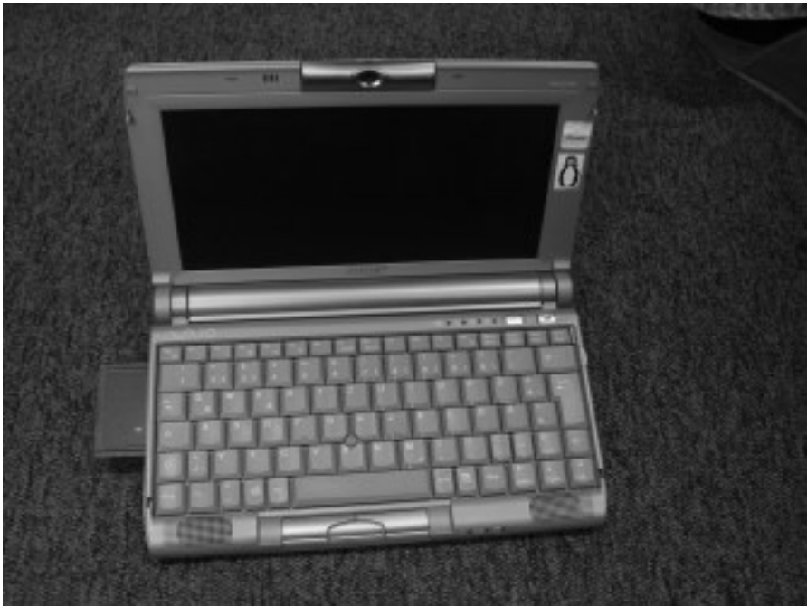
Fig. 7: CMOS camera built into Sony PCG-C1VE Notebook. The camera can be seen at the top of the screen.
