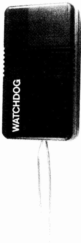
Fig. 5-10 Watchdog-capacitive proximity alarm.
