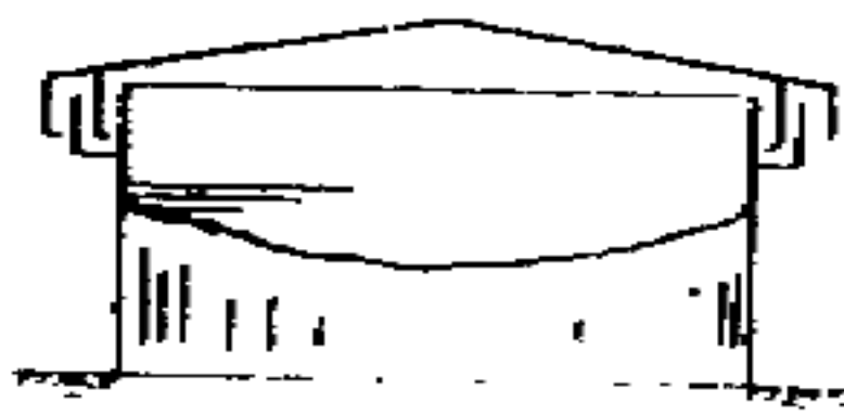
LIFTER ROOF TANK
