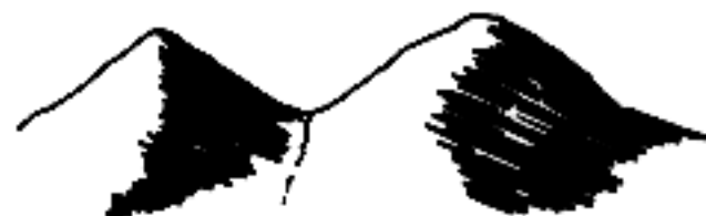
ON GROUND When you are located in a saddle, there is higher ground in two directions and lower ground in two directions
