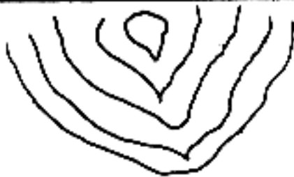
ON MAP U or V shaped contours with the base of the U or V pointing away from higher ground
