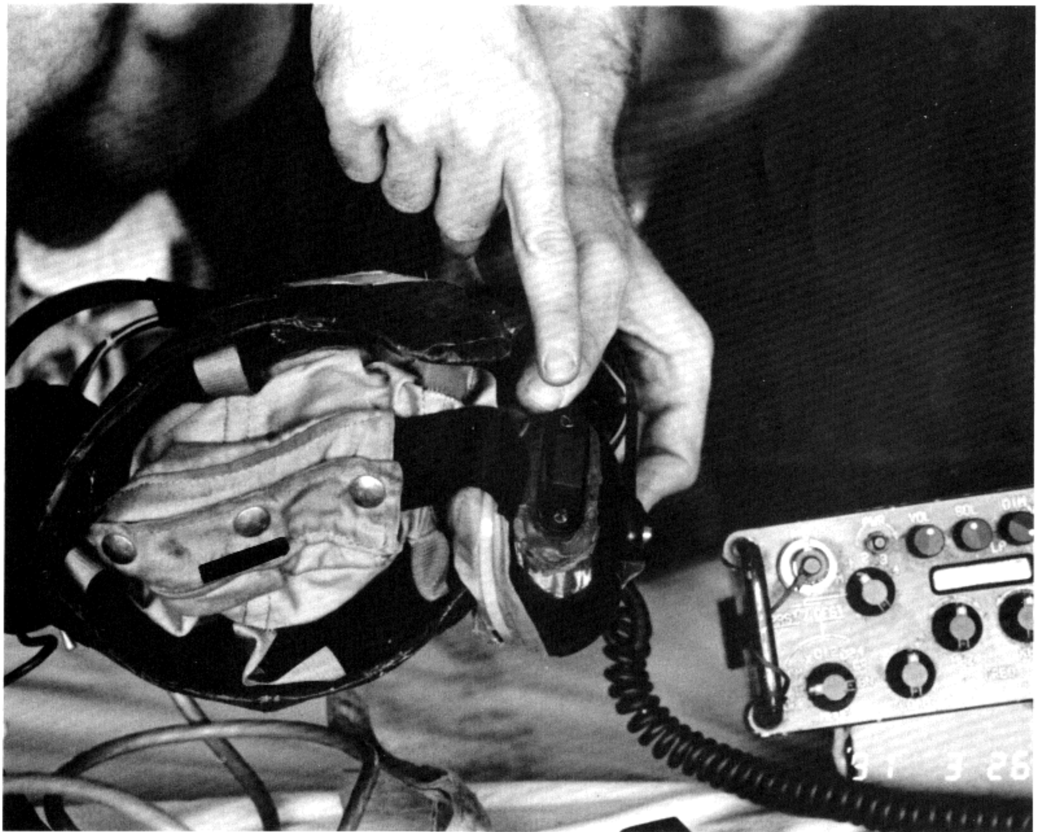
C-2 element communication headset push-to-talk toggle switch (HST-4 sat comm).
