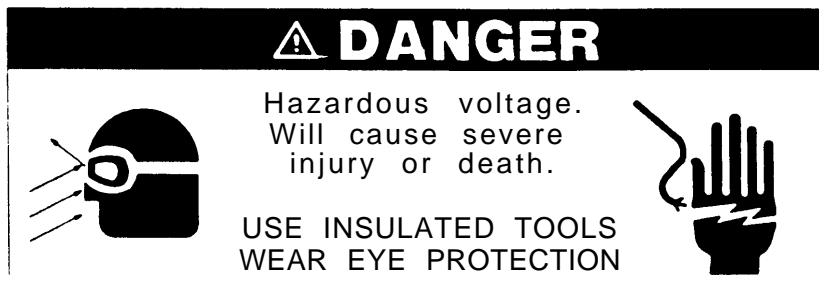
Figure 14-1. Battery warning sign
