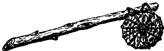
Figure 2-42. Typical pole charge.
