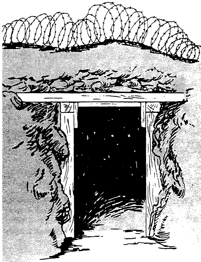
Figure 8-2.—Protective wire on top of overhead cover.
