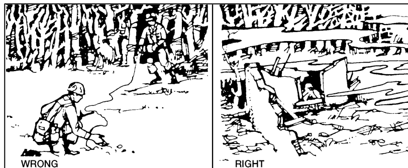
Figure 071-326-5705-2. Camouflage Communication Lines
