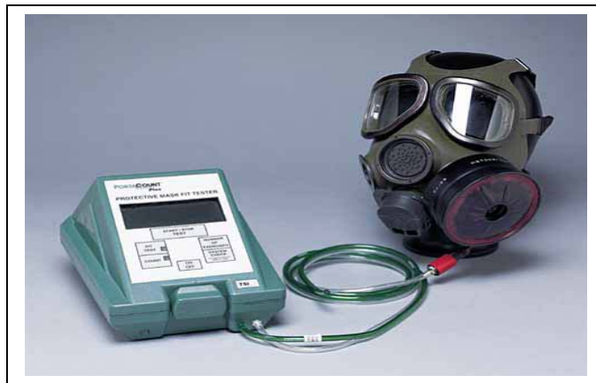
Figure A-6. M41 Protection Assessment Test System
