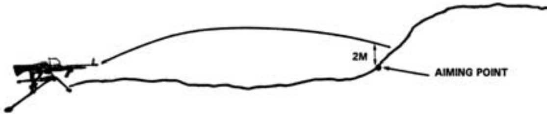
Figure 6-37. Method of Laying When There is a Break in the Uniform Slope (For Ranges Less Than 600 Meters).
