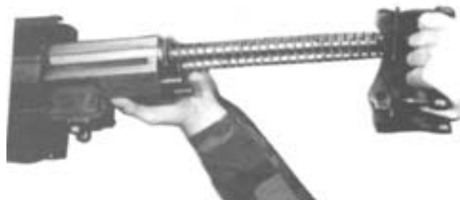
Figure 5-15. Depressing the Sear While Sliding the Bolt Assembly Forward.
