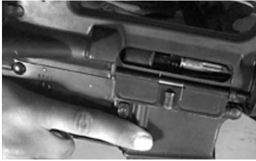
Figure 3-15. Brass Obstructing the Chamber.
