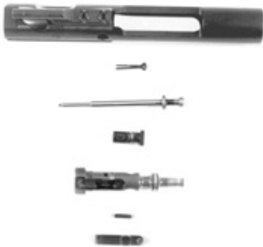
Figure 2-17. Bolt Carrier Disassembled.
