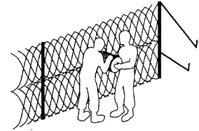
3. Install Top Row And Rack To Rear Horizontal Wire.
