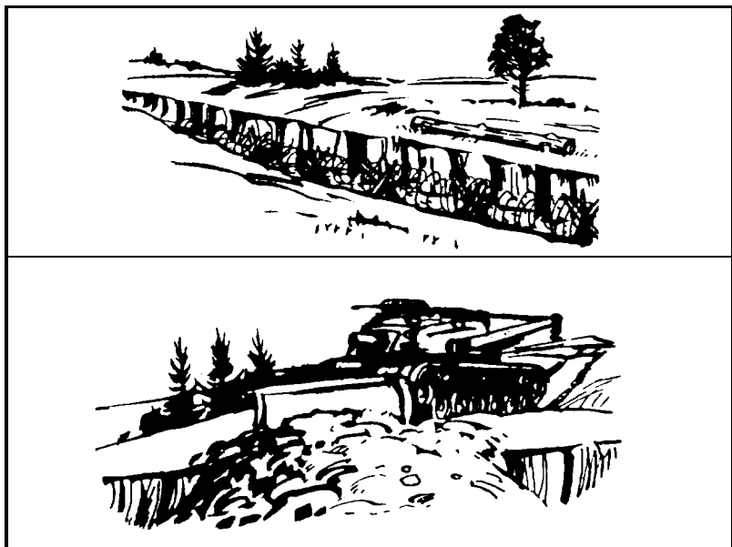
Figure 2-84. Clearing a tank ditch.
