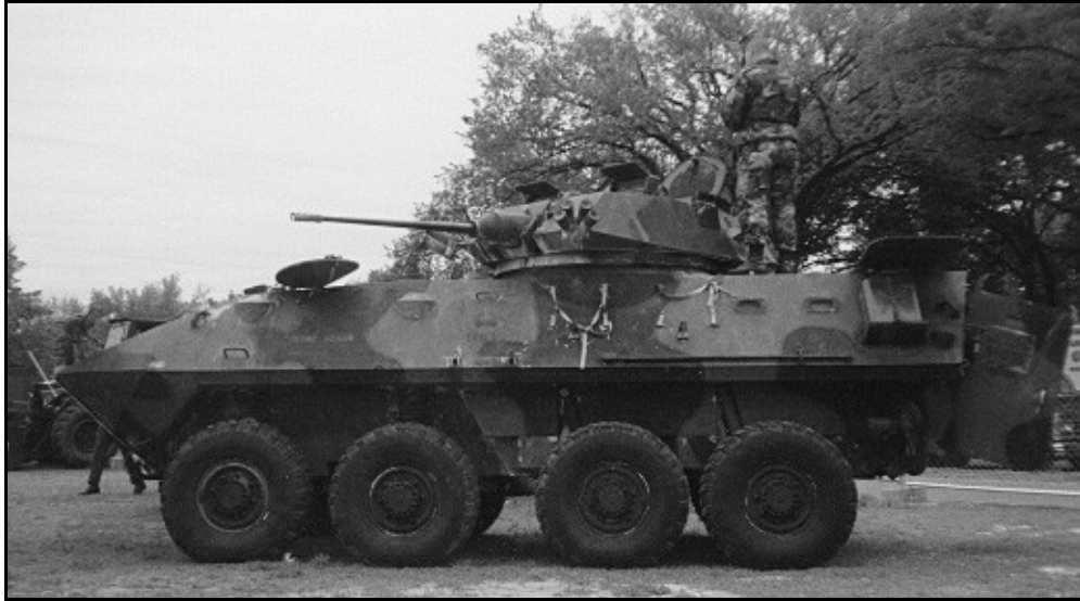
This Light Attack Vehicle (LAV) sports the same main gun as the BFV.
