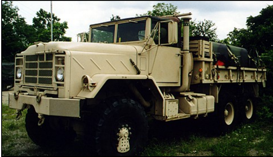
This five ton truck has fuel cells strapped to its back.
