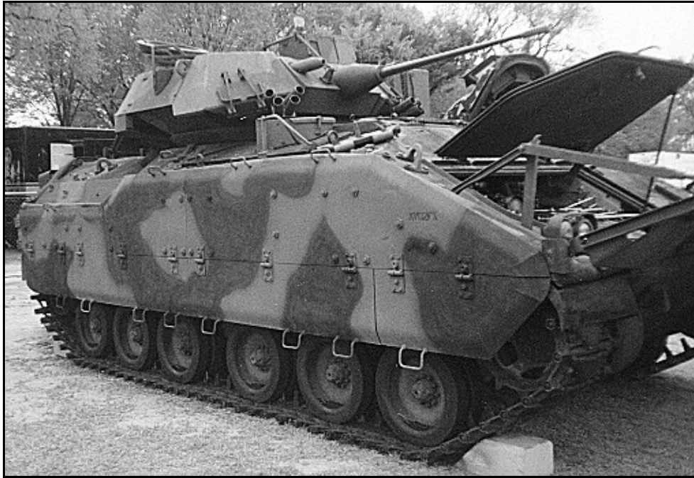
The Bradley Fighting Vehicle, shown with engine access hatch open.
