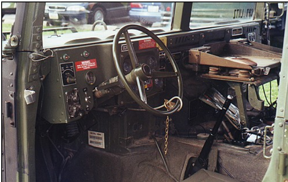
HUMMVEES, like all military trucks, are secured by a simple cable and lock.
