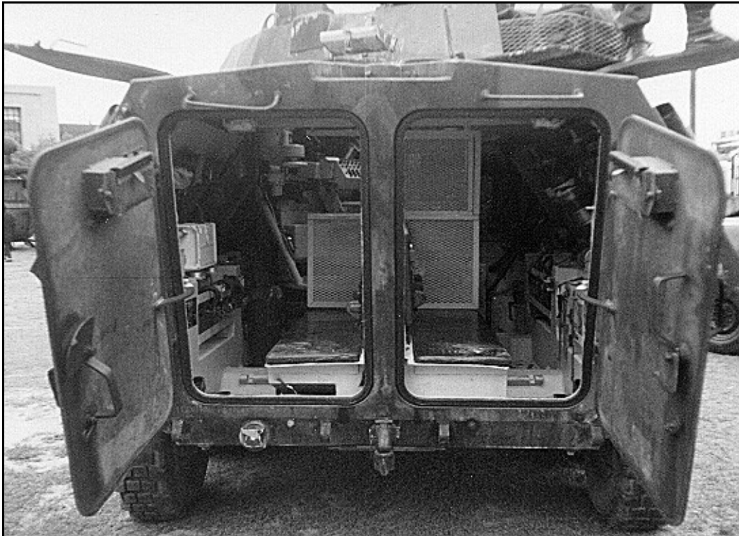
The LAV does not have a ramp; instead it has two manually operated doors.
