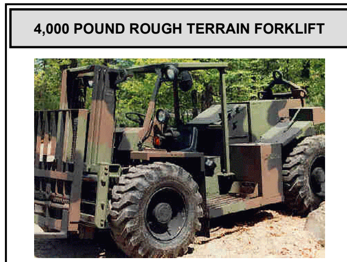
Figure J-4. 4,000 Pound Rough Terrain Forklift
