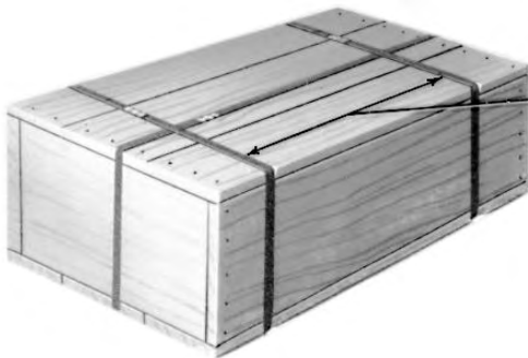
Figure 3-16. Strapping of nailed wood boxes.
