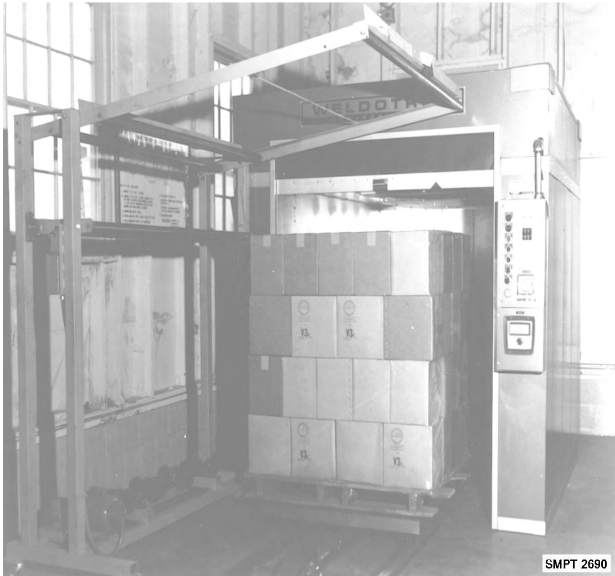
Figure 7-5. Shrink film chamber used for heat shrinking film around palletized load.
