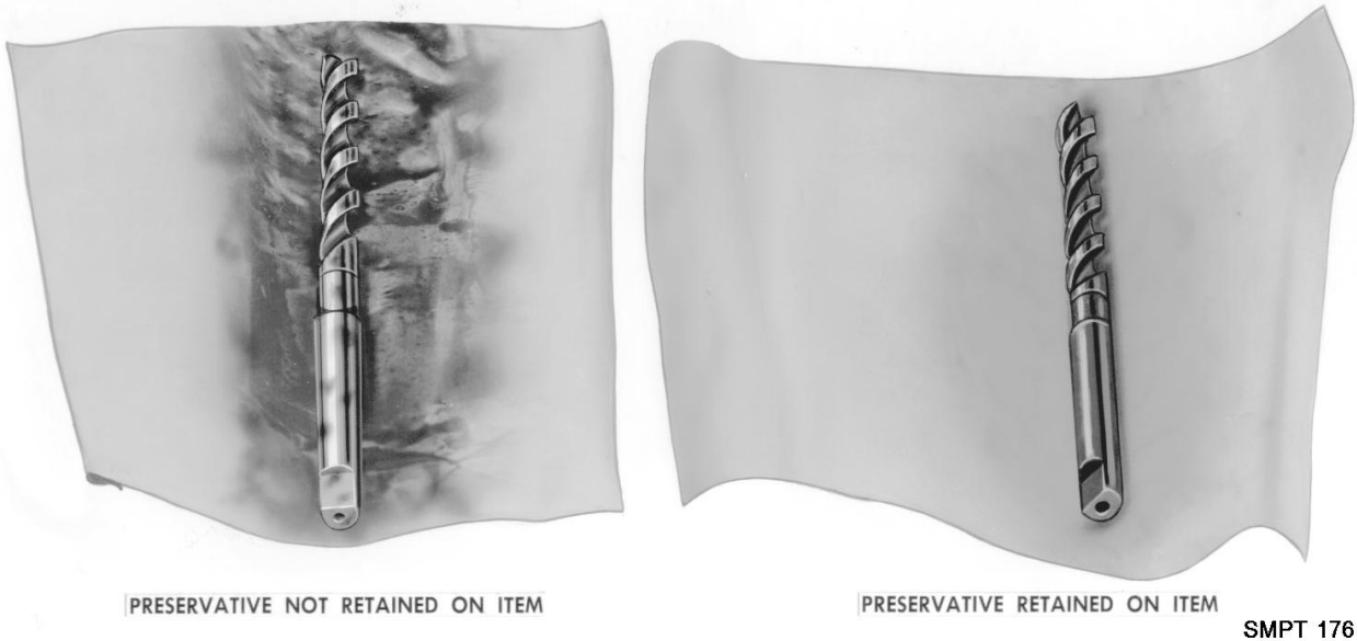
Figure 4-45. Determination of preservative retention.
