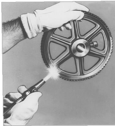
DRYING WITH COMPRESSED AIR
