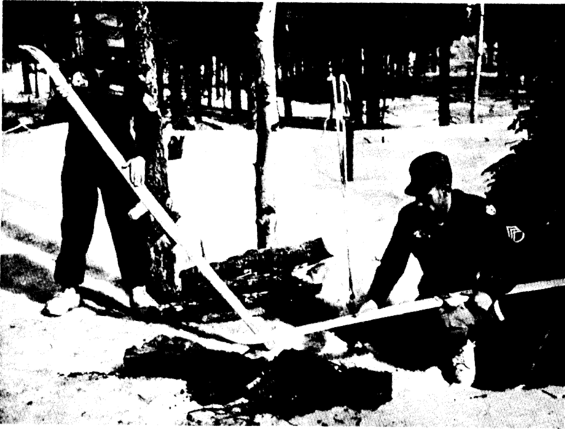
Figure 4-6. Heating skis over an open flame.
