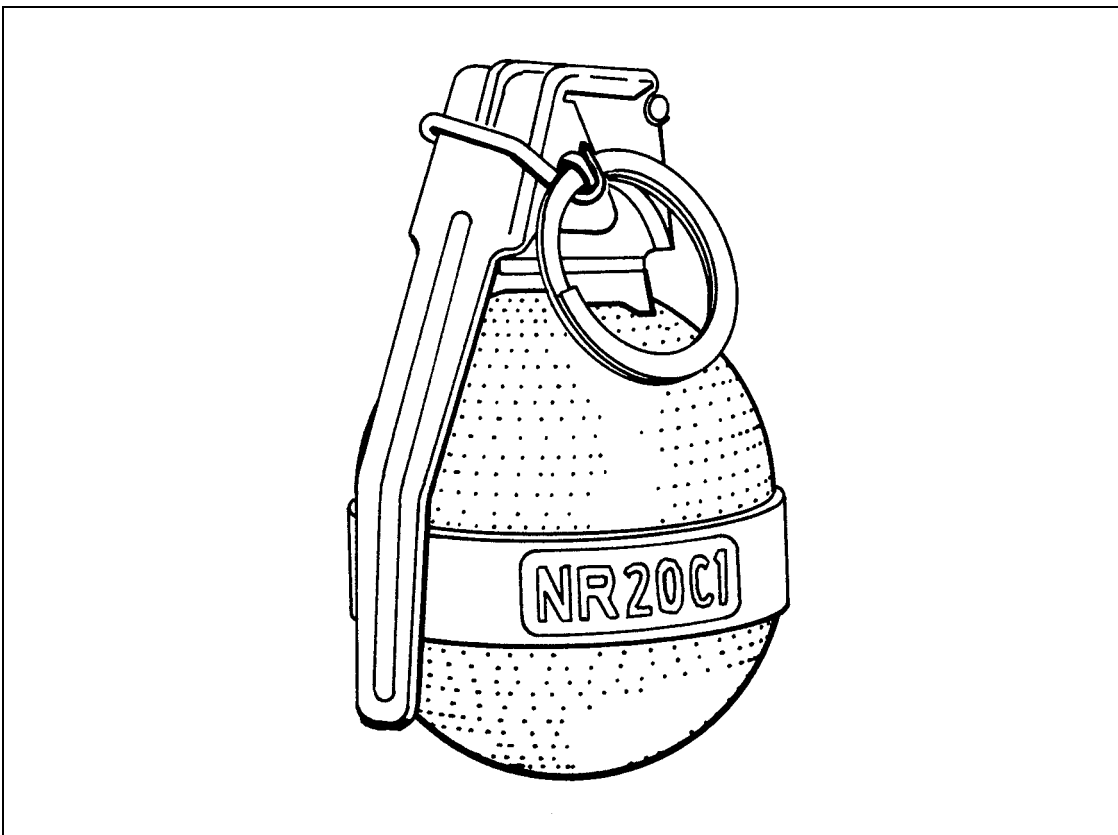
Figure F-8. NR20C1 fragmentation hand grenade.
