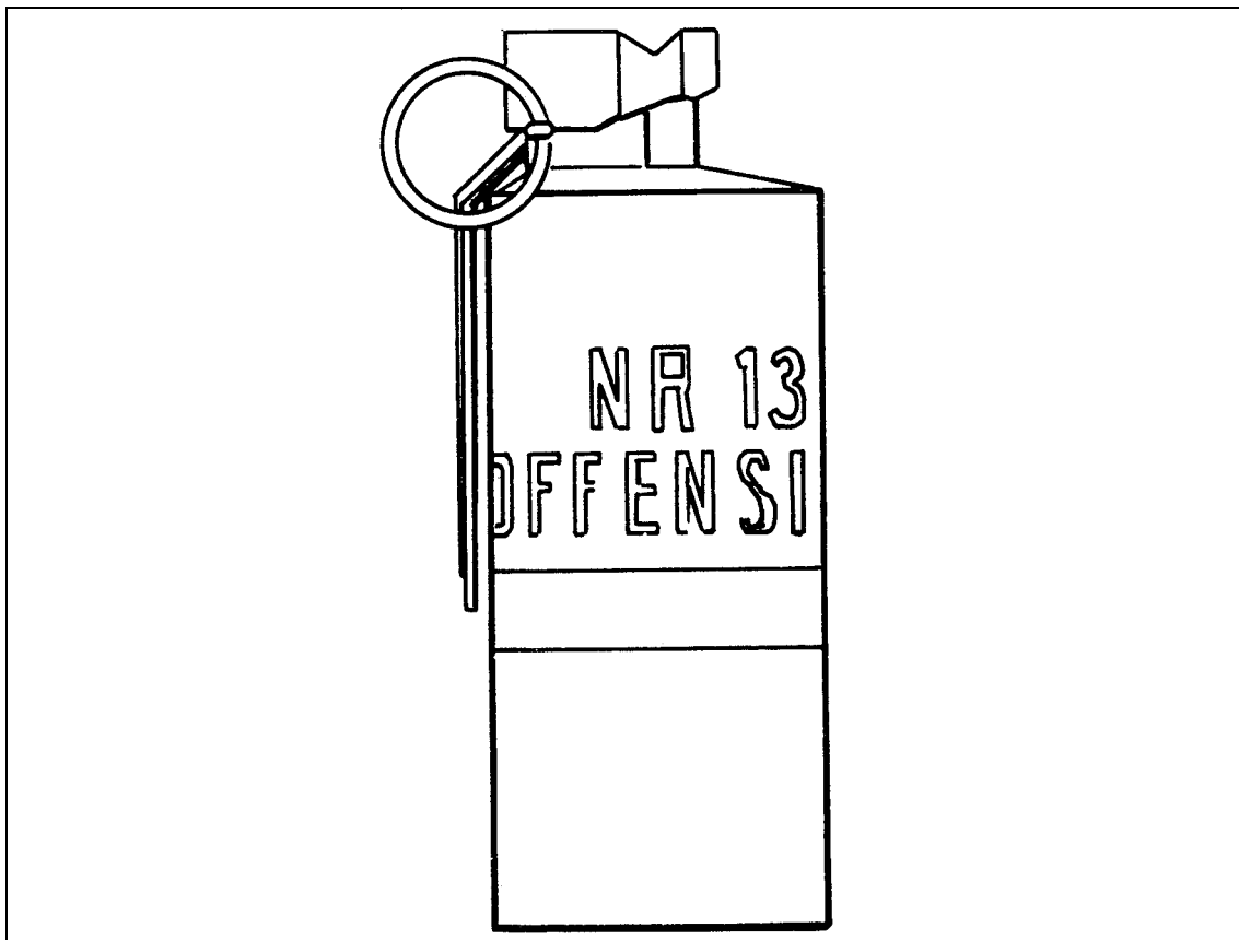
Figure F-2. NR13C1 fragmentation hand grenade.
