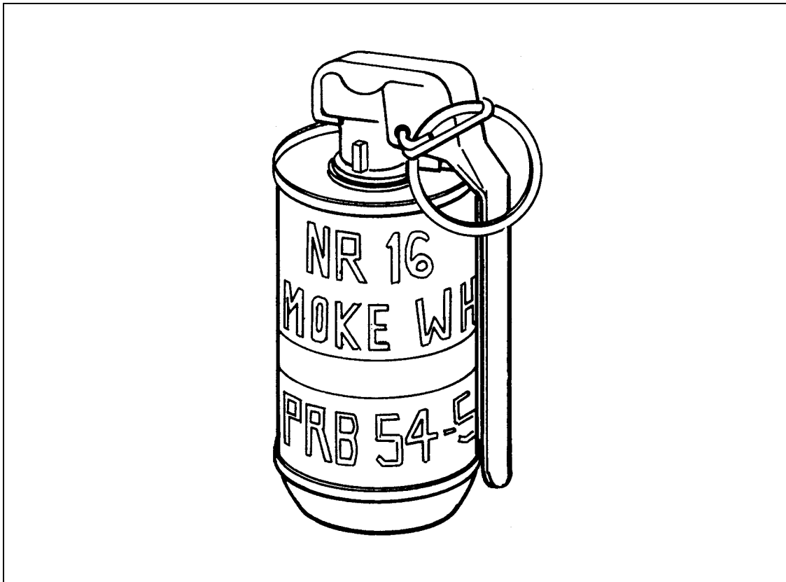
Figure F-7. NR16 smoke hand grenade.
