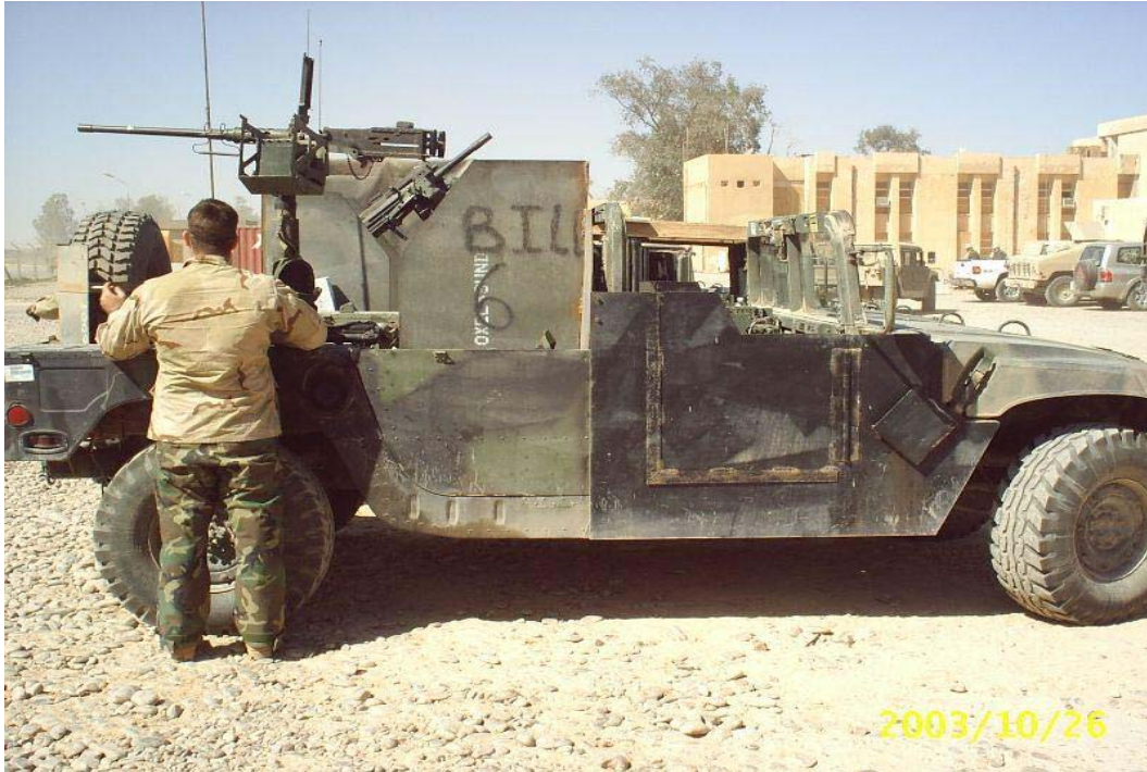
Figure 6-2. Vehicle Hardening and Pedestal Mount
