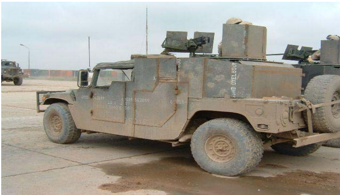
Figure 6-3. Gunner Shields to the Rear and Front
