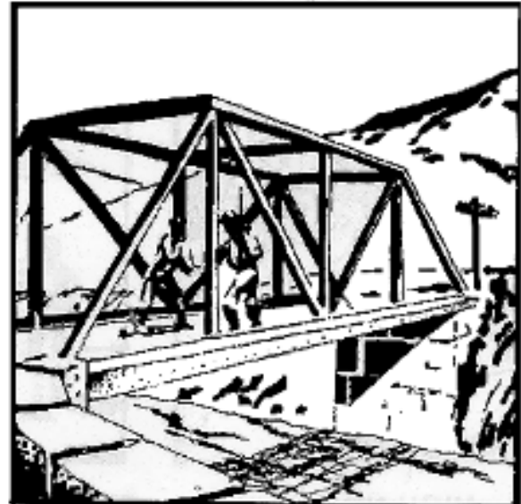
OVERHEAD STEEL BRIDGES
