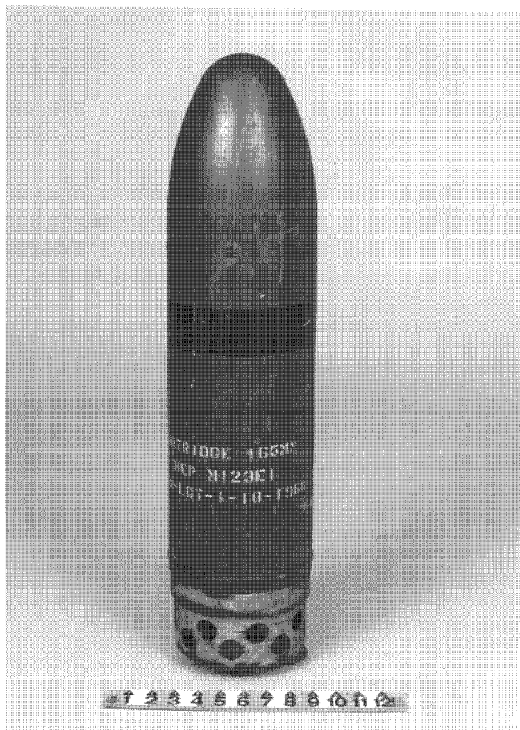
Figure C-6. Spin-stabilized projectile, 165-millimeter HEP.
