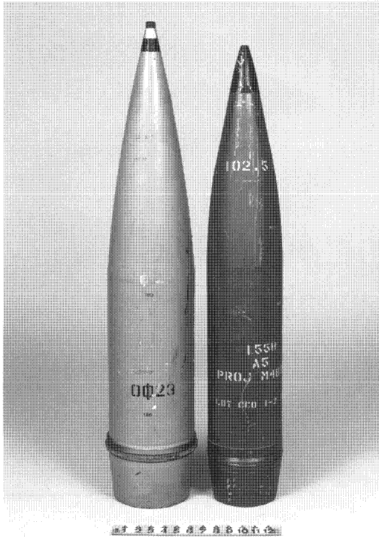
Figure C-4. Spin-stabilized projectiles, 180-millimeter (left) and 155-millimeter (right).
