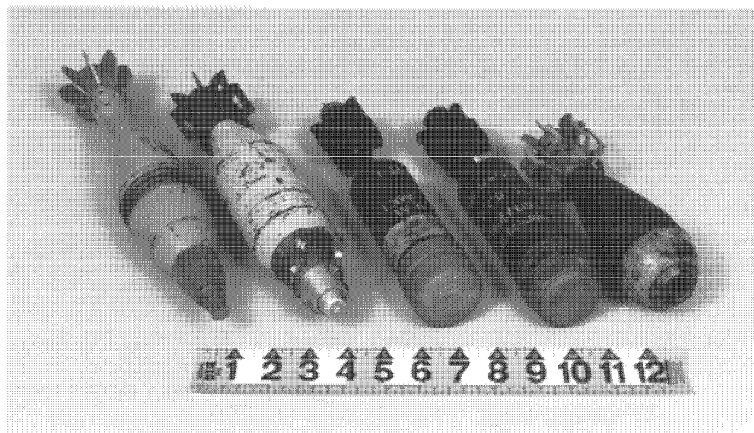
Figure C-10. Fin-stabilized mortars, 60-millimeter and below
