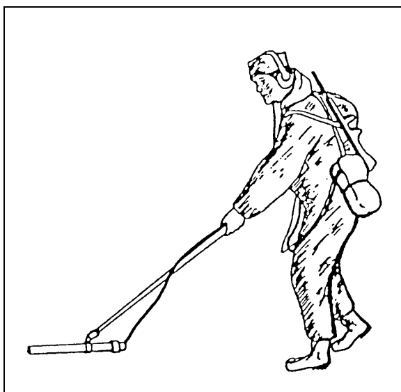
Figure C-10. IMP portable mine detector
