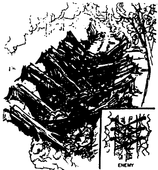
Figure 3-12. Abatis used as a roadblock.
