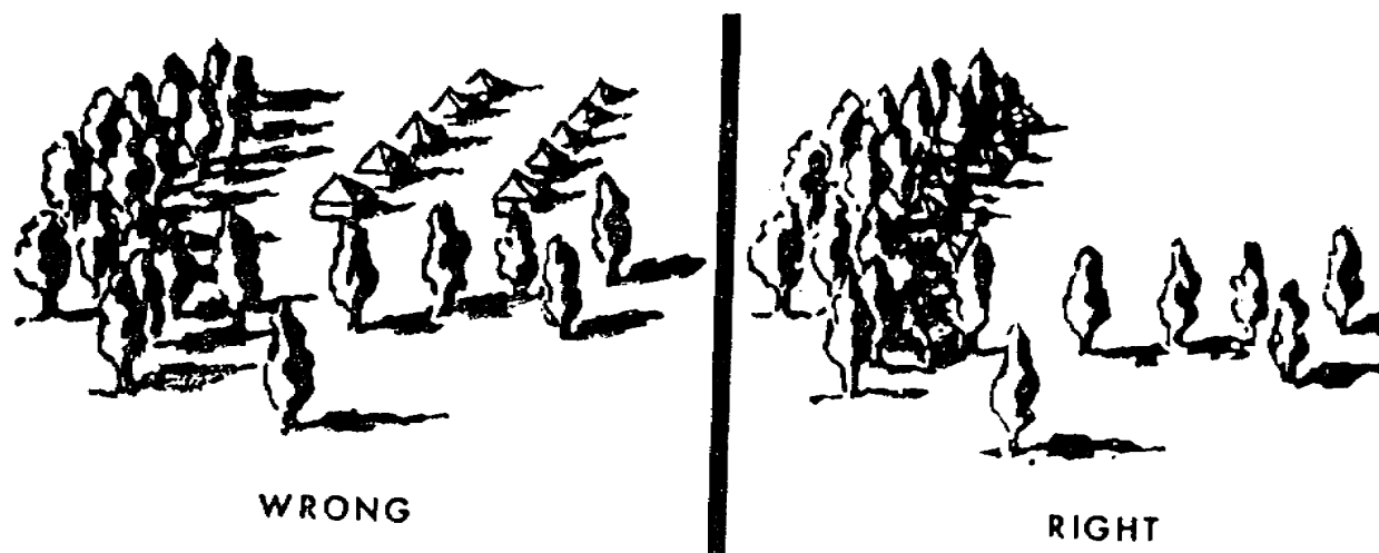
Figure 5-3. Example of proper siting and dispersal of tents in sparsely vegetated terrain (barren).
