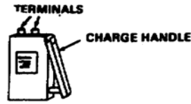
Figure 9. M34 50-cap blasting machine.
