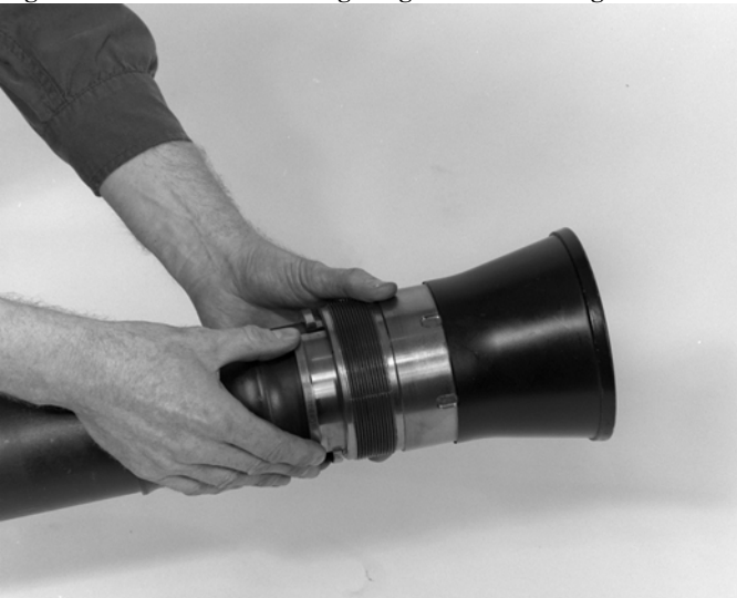
Figure 2-16: Position the Cone on the Muzzle
