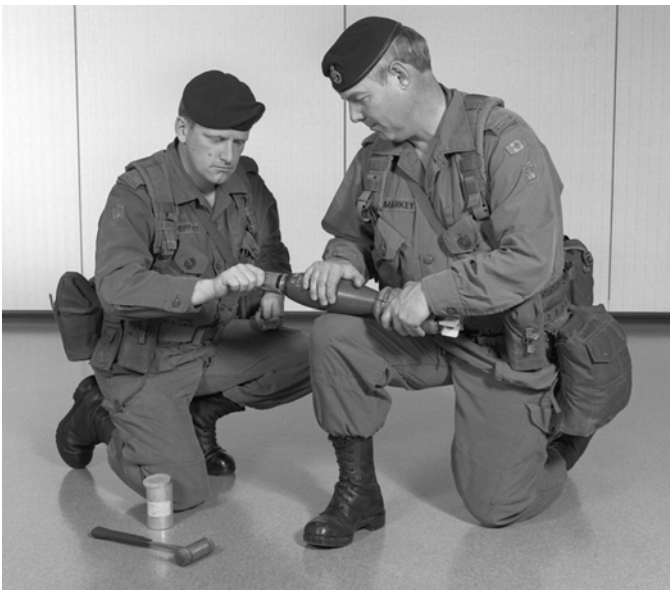
Figure 3-11: Insert Fuze PPD 323 Clockwise by Hand
