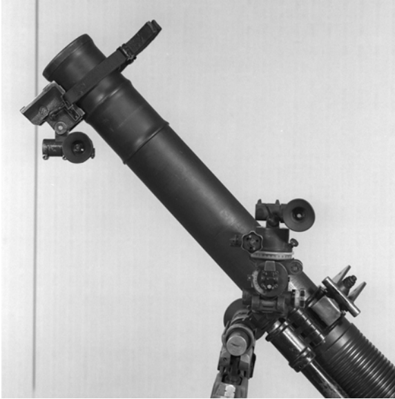
Figure 4-13: Boresight Mounted on Bottom of the Barrel
