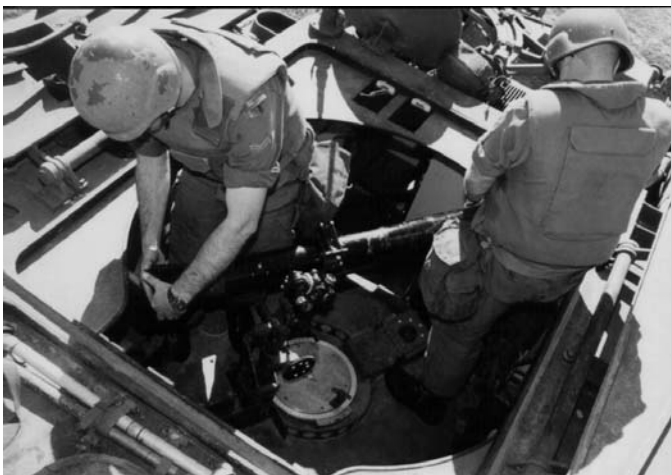
Figure 6-7: Misfire Drills—Removing the Firing Pin
