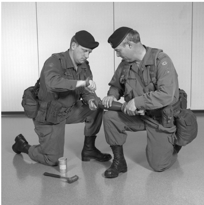
Figure 3-12: Tighten the PPD 323 Fuze
