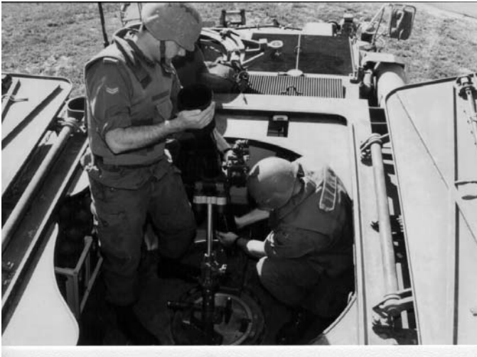
Figure 6-6: Misfire Drills—Gaining Access to the Firing Pin
