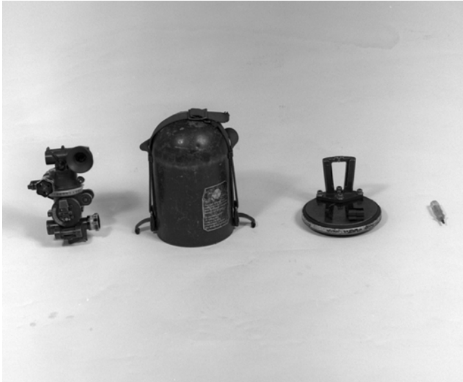
Figure 2-8: Sight Unit C2A1 and Case
