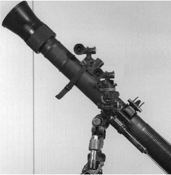
Figure 4-14: Boresight Mounted for Testing Elevation and Bearing
