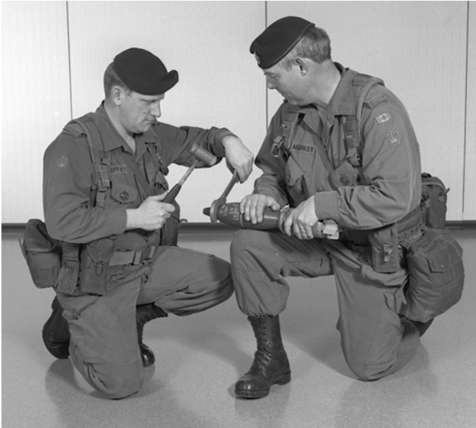
Figure 3-10: Remove Fuze PD DM 111A3/A4
