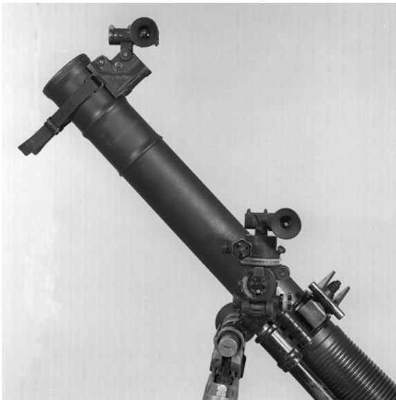
Figure 4-12: Boresight Mounted on Top of the Barrel
