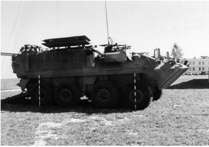
Figure 6-10: Baseplate Re-occupation—Vehicle Referencing Stakes
