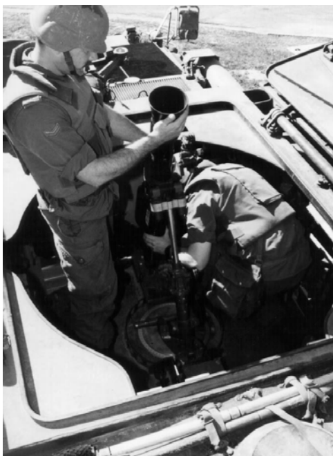
Figure 6-8: Misfire Drills—Tipping up the Mortar
