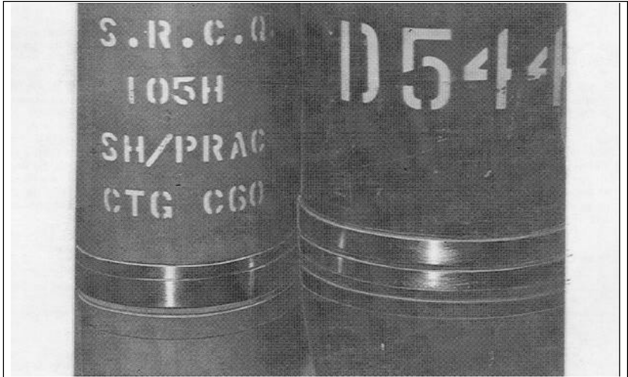
Figure 9-5-2 Typical Driving Bands
