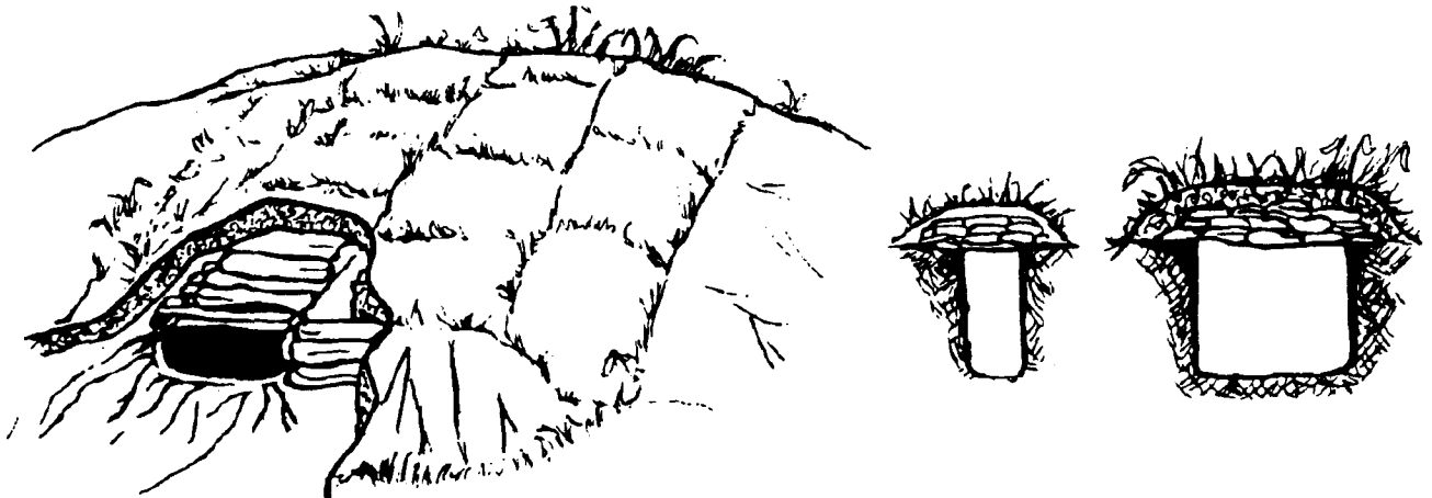
Figure 4-6. Sandbags protected with sod and earth cover.
