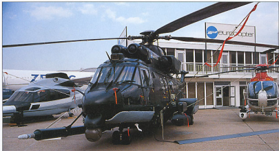
Eurocopter AS 332A2 Cougar rescue version with in-flight refuelling probe
