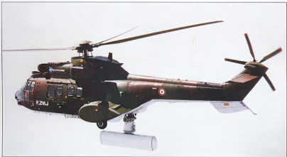
Eurocopter AS 532 UL Cougar Mk 1 with Horizon battlefield surveillance system
