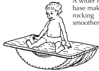
For the rocker, you can use 2 pieces of old tire.
