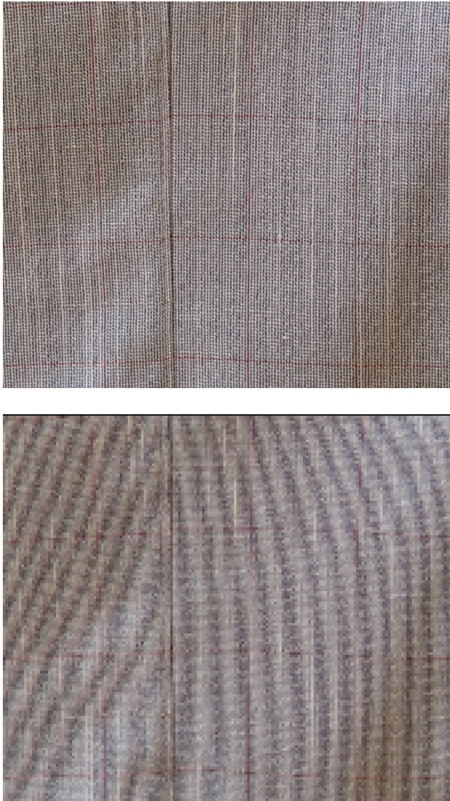
Figure 4.35 Two images that are representations of the same pattern on a jacket as seen with two different image sensor resolutions. Note pronounced aliasing effect in image on the bottom.
