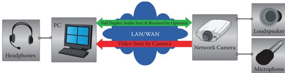
Figure 6.6 In full-duplex mode, audio is sent to and from the operator simultaneously.
