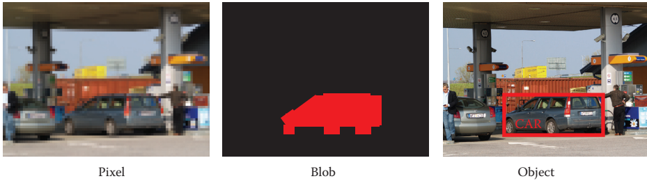
Figure 14.1 IV applications are based on detecting and tracking pixels, blobs, or objects.
