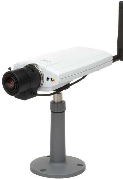
Figure 9.1 A network camera with built-in wireless networking — in this case, 802.11b/g.
