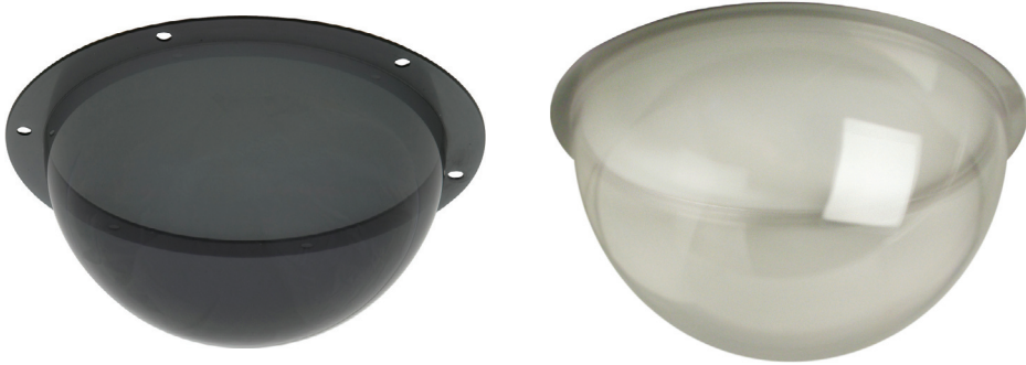
Figure 15.8 Examples of a clear and a smoked bubble for a PTZ dome camera. Although the smoked bubble makes it difficult to see in which direction the camera is positioned, it also reduces the amount of light and therefore the image quality.
