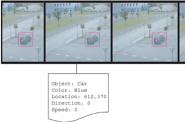
Figure 13.7 A video stream tagged with metadata — for example, the object, color, and location of a car parked in a parking lot.
