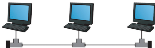
Figure 8.6 Ethernet 10BASE2 cabling may still be used in some older installations, but not in new installations today.
