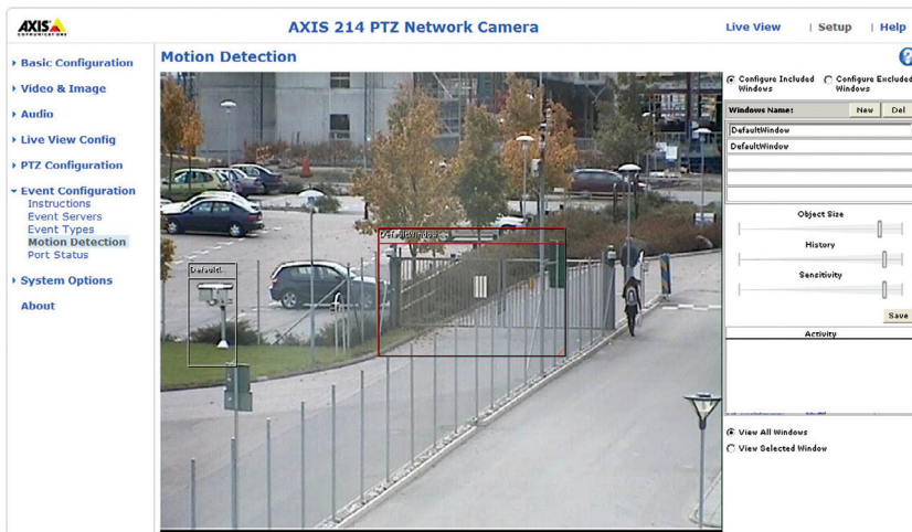
Figure 14.2 Advanced VMD functionality in network cameras includes the option of setting up several VMD windows, which then can be defined individually based on adjustable parameters such as object size, history, and sensitivity.
