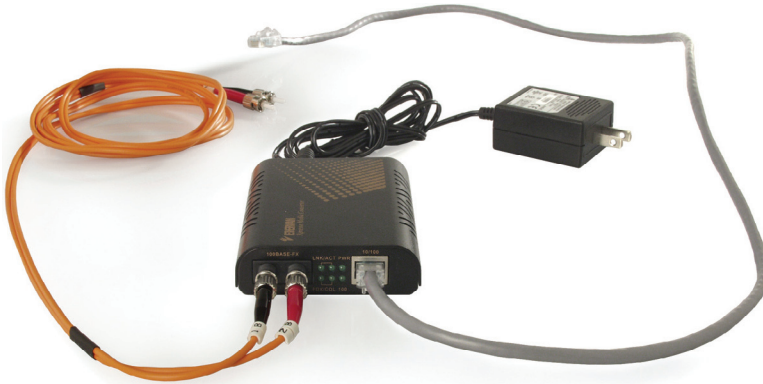
Figure 8.8 A media converter, also called a fiber transceiver, can be used to connect any device with an RJ-45 plug (e.g., a network camera) to a fiber network.
