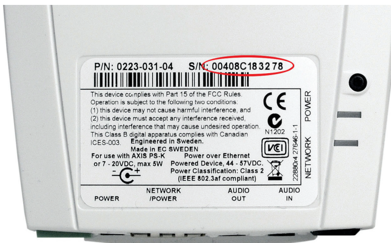
Figure 8.9 Each networking device has a unique MAC address, which is often found on the product label. In this photo, it is shown as the serial number (S/N).
