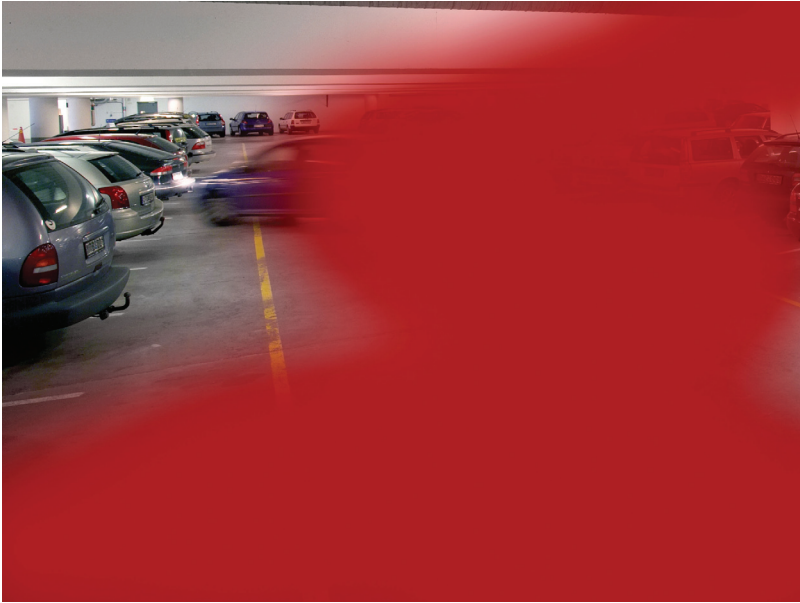
Figure 14.3 Camera tampering detection will (within seconds) detect if a camera has been repositioned, is out of focus, or has been covered.
