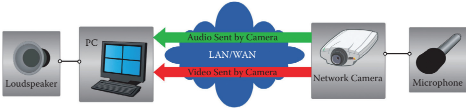
Figure 6.3 In simplex mode, audio is sent in one direction only. In this case, the camera sends audio to the operator.
