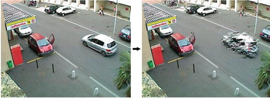
Figure 14.20 An illustration of privacy masking where only the provision of the right password can undo the masking. (Picture courtesy of EMITALL Surveillance SA.)
