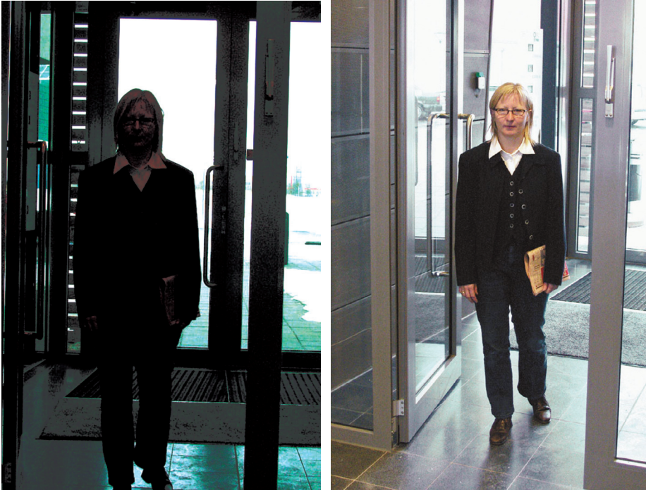
Figure 15.4 (Left) Avoid very bright areas in an image by changing the camera position. (Right) Advanced cameras include a feature that compensates for backlight.
