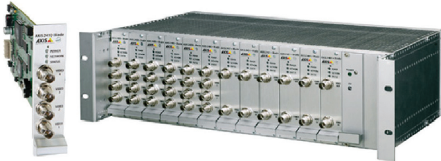
Figure 7.7 Photograph of a blade video encoder (at left) and a 3U video encoder rack (at right). A 3U video encoder rack can hold as many as 48 channels, providing high density and saving on rack space. If a blade needs replacement, having hot-swapping capabilities means that only four analog channels will be down for a short time.
