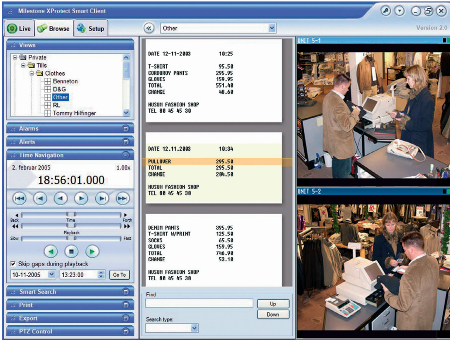
Figure 12.21 An example of a PoS system integrated with video surveillance. (Picture courtesy of Milestone Systems.)
