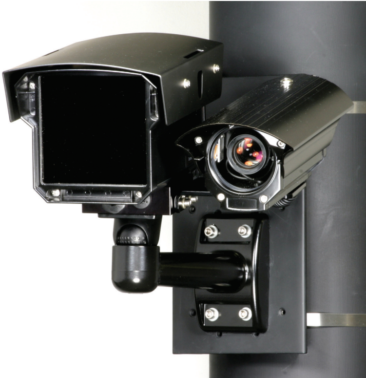
Figure 14.18 In an ANPR application, specialty cameras are often used to ensure that a clear capture of the number plate can be provided at all times of the day. A second camera can be used to provide an overview image of the car. (Picture courtesy of Extreme CCTV.)
