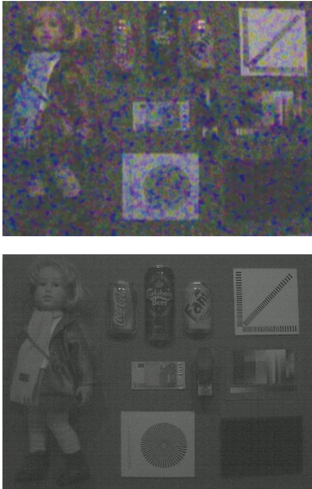
Figure 4.4 Images were taken with two similarly priced network cameras from brand-name vendors under a lighting condition of 1 lux. The image on the bottom clearly looks better. The image on the top, however, was from a camera that was specified to have the lower light sensitivity level, 0.8 lux versus 1 lux.
