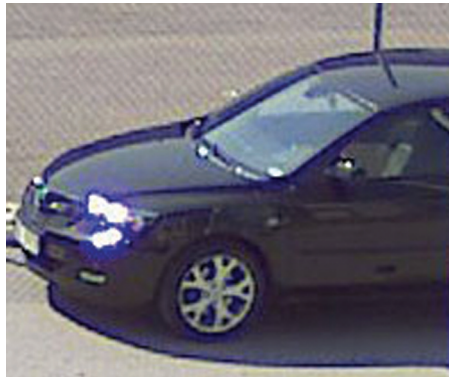
Figure 3.22 Images using a network camera with 1280×1024 or 1.3-megapixel resolution. Same area of coverage. More details can be seen in an image from a megapixel camera because it offers three to four times higher pixel resolution than an image from a non-megapixel camera (Figure 3.21).
