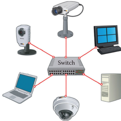
Figure 8.4 In a star topology, all nodes connect to a central point.
