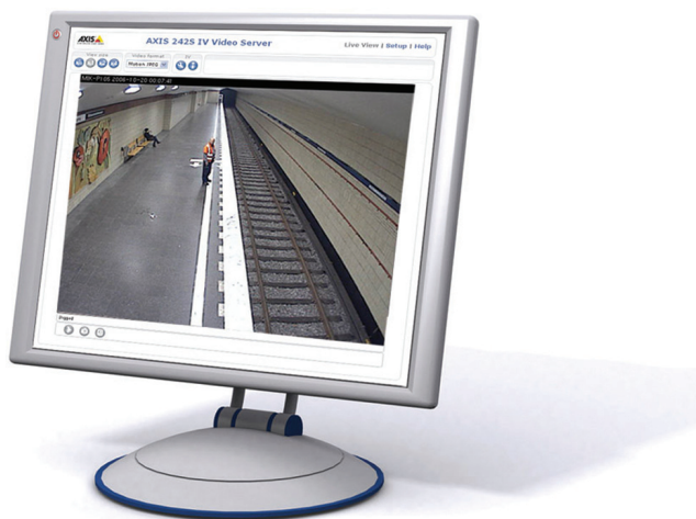
Figure 14.13 Virtual fence can be used to detect and send an alert if someone enters the rail or subway track.
