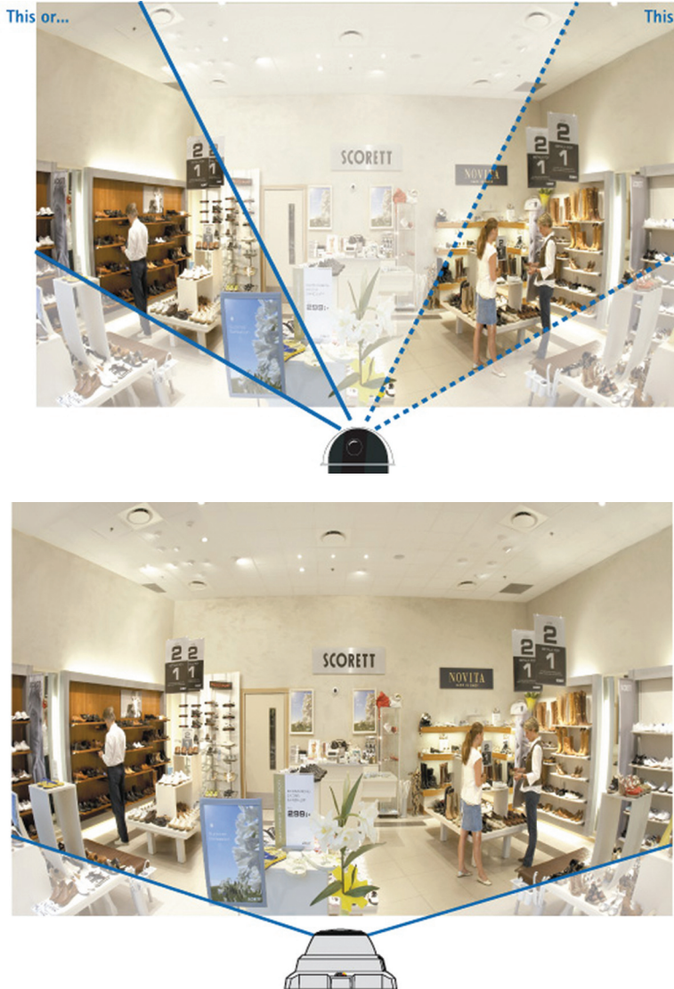
Figure 3.15 A conventional PTZ camera can cover a bigger area but it can only see a small part at the same time (top), whereas a nonmechanical-PTZ camera sees the entire monitored area (bottom).
