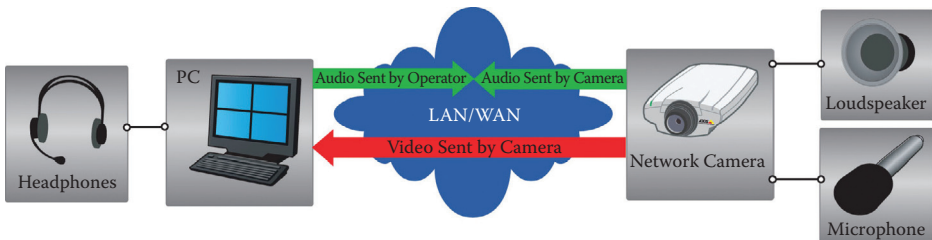
Figure 6.5 In half-duplex mode, audio is sent in both directions, but only one party at a time can send.
