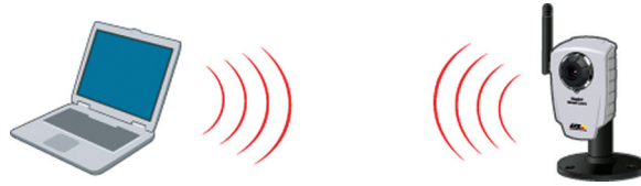
Figure 9.7 A network camera with built-in 802.11b/g can be set to work in ad hoc mode. This is, however, not very common and not recommended.
