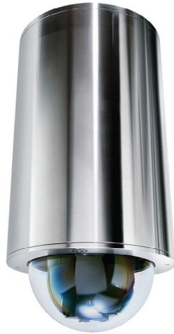
Figure 15.20 Example dome camera and housing unit designed and certified for use in potentially explosive atmospheres and harsh environmental conditions. The camera housing is made of stainless steel and thus is ideally suited for use in offshore and onshore environments. Stainless steel screws and mounting bracket are incorporated, ensuring a totally corrosion-free unit. (Courtesy of Dexter, Dutch Explosafety Center.)
