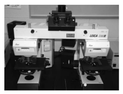
**FIGURE S.13A** Comparison microscope used to compare latent fingerprints lifted from crime scene to suspect's fingerprint cards.
