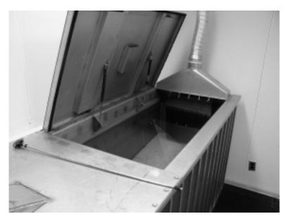
**FIGURE B.9** A metal tank filled with water allowing the firearm examiner to recover bullets from the test firing of handguns.
