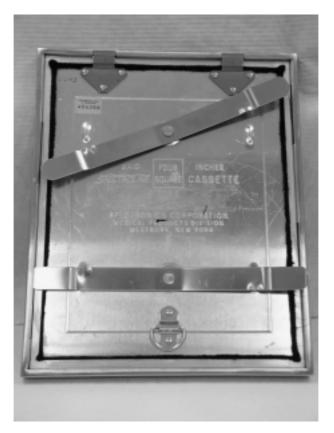
FIGURE C.4 A metal case that is lightproof. It is used for the development of the autoradiograph.
