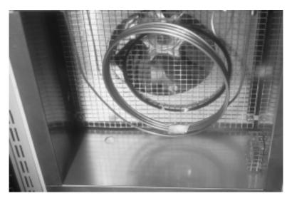
FIGURE P.1 Inert material packed into capillary columns used in gas chromatography.
