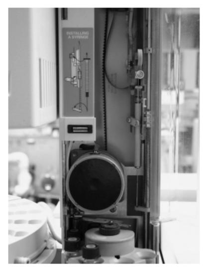
**FIGURE 1.4** Injection port uses a syringe to automatically aspirate the sample from the vial and inject the sample into the column of the GC/MS instrument.
