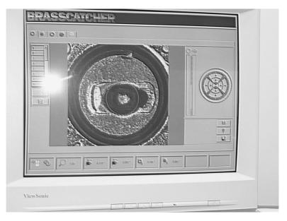
FIGURE F.5 The use of the IBIS for identifying a firing pin impression.
