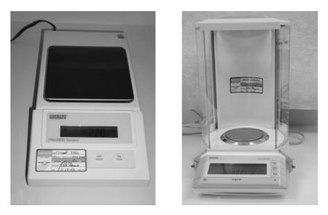
**FIGURE A.3** Analytical balances used for measuring reagents, dry chemicals, and for measuring the accuracy of manual pipettes (the amount of fluid dispensed).
