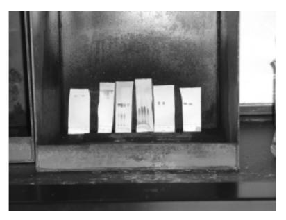
**FIGURE C.15** The separation of drugs that have been spotted on thin-layer silica plates. Special chemical sprays that produce a color reaction are applied to the plates. This method of separation is performed inside a spraying chamber.
