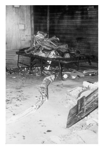
**FIGURE A.6B** Material used to make a fire trail, and debris piled in the corner of a room to ensure an intense fire.
