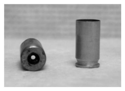
**FIGURE C.3** Firearm cartridge in which the primer compound is contained in a centrally positioned primer cap.
