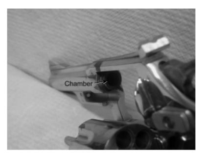
FIGURE C.11 Cylinder chambers.
