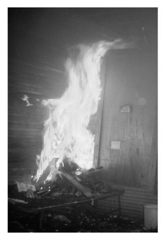
FIGURE A.5A Debris placed in a corner of a room to enhance the fire's intensity.
