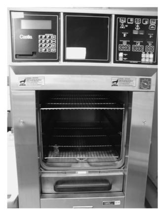
**FIGURE A.10** An enclosed chamber for the sterilization under pressure of laboratory glassware, instruments, plastic tubes, etc.
