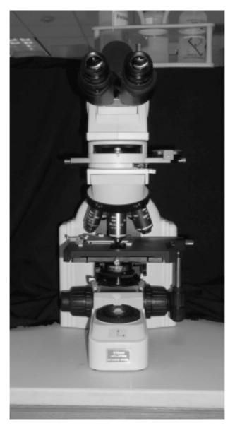
FIGURE P.11 Polarized light microscope with polarizing filters.
