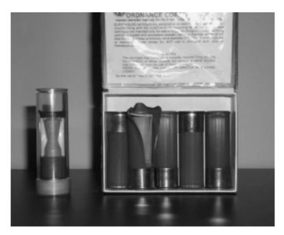
FIGURE W.1 Gunshot cartridges showing the wading material inside.
