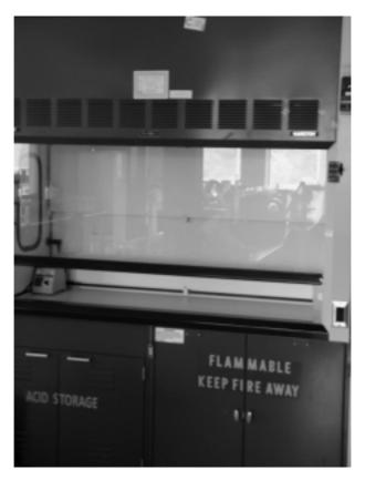
FIGURE F.9 Fume hood used for safe handling of chemicals and other hazardous materials.
