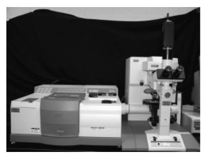
**FIGURE F.8** Typical FT–IR micro imaging configuration. The FT–IR instrument is used for the nondestructive acquisition of molecular spectra from various forensic samples.
