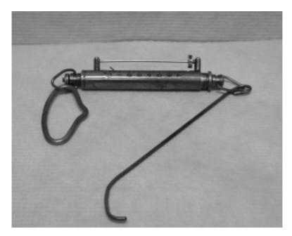
FIGURE T.9A Trigger pull gauge.
