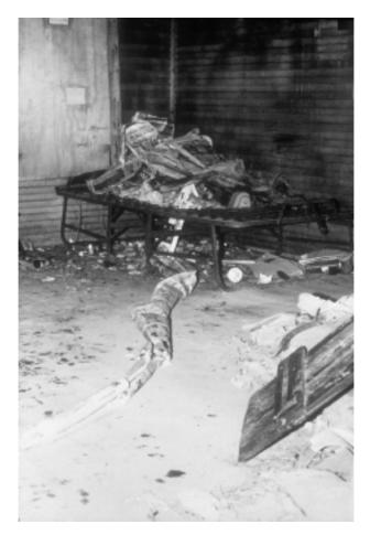
FIGURE T.8A Paper and debris used as trailer, allowing the fire to follow a certain direction.
