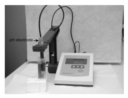
FIGURE P.4 pH electrode attached to pH meter.
