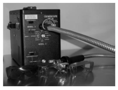
**FIGURE C.22** An alternate light source made by SPEX<sup>®</sup> uses different wavelengths of light. With special color glasses one can observe various types of stains found on evidence.
