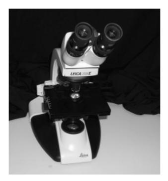
FIGURE M.10 Transmitted-light compound microscope.
