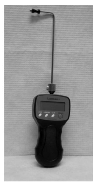
FIGURE T.9B A handheld trigger pull gauge wih a digital readout.
