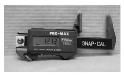
**FIGURE V.1** Vernier caliper with a digital display. Used by firearm examiners to measure the gauge of a firearm.
