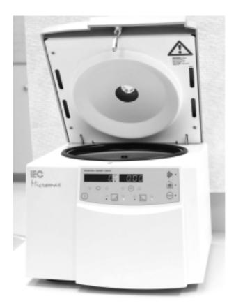
**FIGURE C.7** A rotary machine with accessory containers, tubes, and rotors for the separation by controlled centrifugal force of substances having different densities.
