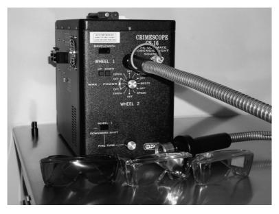
FIGURE A.1 An alternate light source manufactured by SPEX®.
