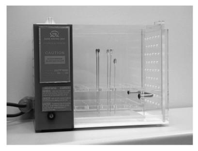
**FIGURE S.18** A container for storing wet swabs. Air is then circulated through the container, which will allow the swabs to air dry. The container prevents contamination of the swabs as they are drying.
