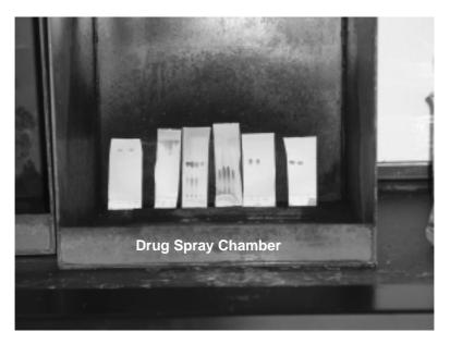
**FIGURE C.12** Spraying chamber for developing thin-layer chromatograph (TLC) plates in drug chemistry.
