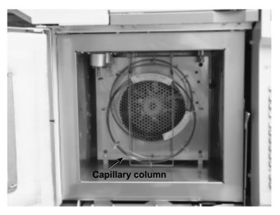
**FIGURE C.1** A narrow-bore glass tube that is found inside a gas chromatography instrument. This is where the separation of the chemical compounds takes place.
