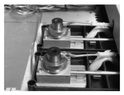
FIGURE F.6 Two-flame ionization detector (FID) inside a gas chromatograph instrument.
