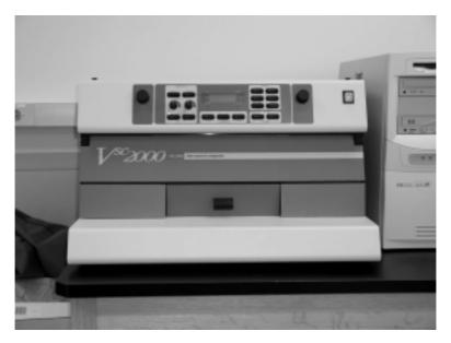
FIGURE V.2 Video spectral comparator.
