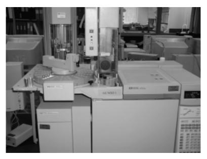
**FIGURE G.5** GC/MS instrument. The gas chromatography (GC) instrument separates the compounds, and the mass spectroscopy (MS) provides information concerning the chemical properties of each of the compounds as it elutes from the chromatographic column.
