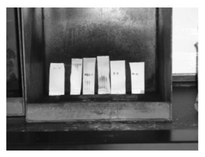
FIGURE T.4 Drug chemistry spraying chamber on TLC plates.
