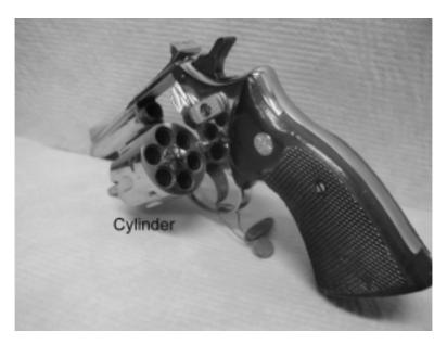
FIGURE C.23 The revolving cylinder contains six firing chambers, each able to accommodate a single cartridge.
