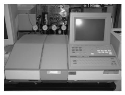
**FIGURE 1.3** Infrared spectrophotometry instrument. The spectra from the IR instrument are referred to as "fingerprint spectra" of a compound, which aids in classification of the chemical.
