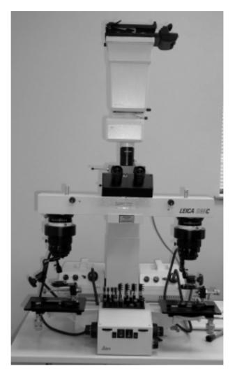
**FIGURE C.17** A firearms examiner's (ballistics) comparison microscope. It has an optical bridge, separate objectives, dual focusing stages, specimen holders, and two illuminators, the angles and intensities of which are independently adjustable.
