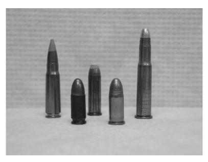
FIGURE A.2 Various types of ammunition that can be found in firearm examinations.
