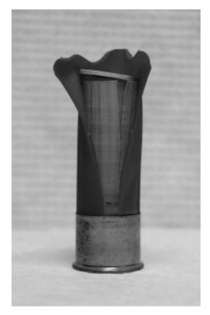
FIGURE S.5A Opening of a shotshell showing the inside.
