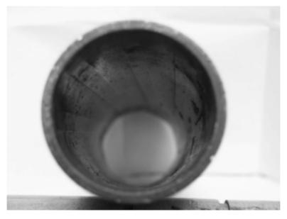
**FIGURE L.1A** Looking down through a section of a barrel, the cuttings in the barrel are referred to as the lands and grooves.
