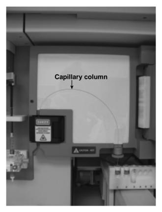
**FIGURE C.2** Capillary electrophoresis is used to separate DNA fragments; a liquid polymer flows through the capillary along with different sized DNA fragments.
