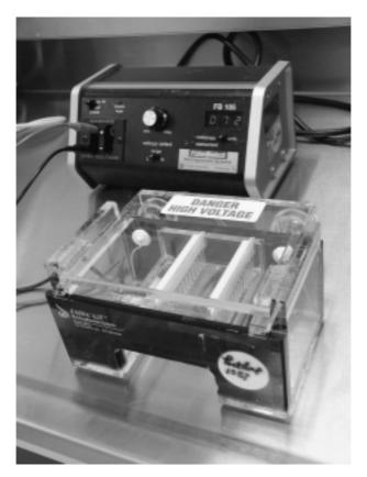
FIGURE E.3 Electrophoresis setup showing gel chamber with plastic combs and a power supply.
