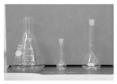
FIGURE V.3 Different sizes and shapes of volumetric flasks.
