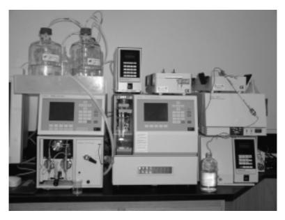
**FIGURE L.4** The LCMS utilizes a closed system and pumps to pressurize the solvent (mobile phase) and to force the liquid through the column.
