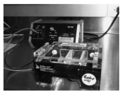
FIGURE G.6 Gel electrophoresis unit with power supply unit.
