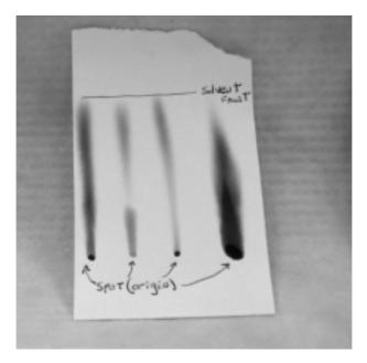
**FIGURE S.6** Different types of markers spotted on filter paper, which is placed into a jar containing a solvent. Once the filter paper is removed from the jar the solvent front (where the chemical reagent solution stops) is noticed at the top of the filter paper.
