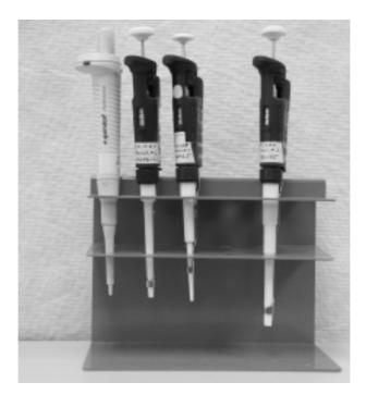
**FIGURE M.7** Handheld mechanical pipettes that can deliver a specific volume of liquid. Each pippette contains an adjustable dial that can be set for a specific volume measured in microliters.
