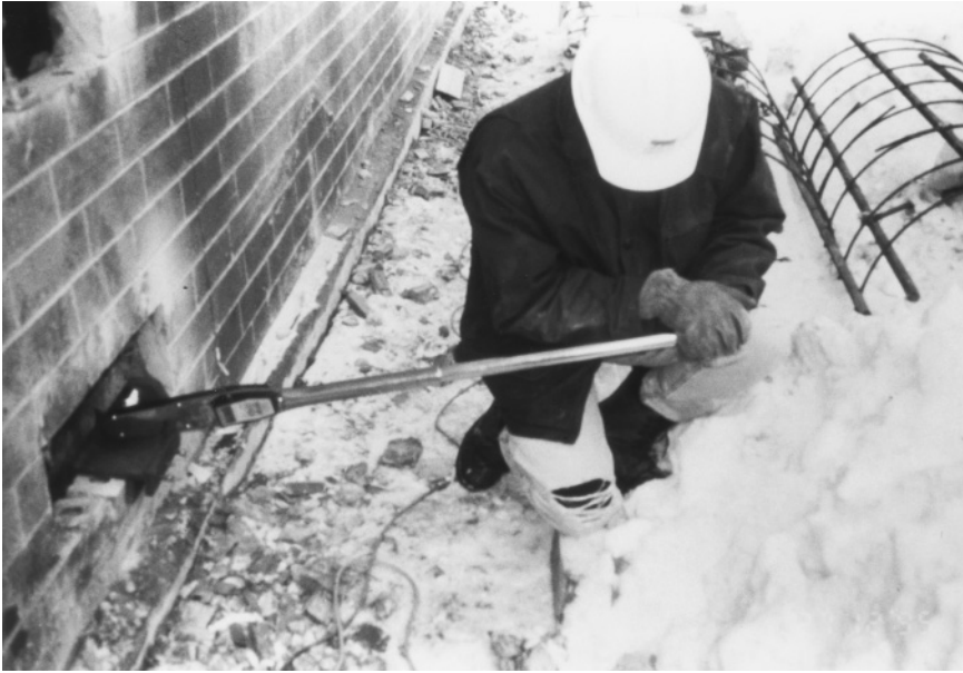
Figure 8.15 Bond-wrench testing on in situ brick masonry.
