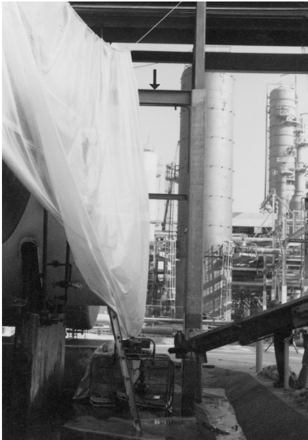
Figure 4.5 Fallen aerial platform basket. The basket separated from its boom connection after coming into contact with the cross beam at the arrow.
