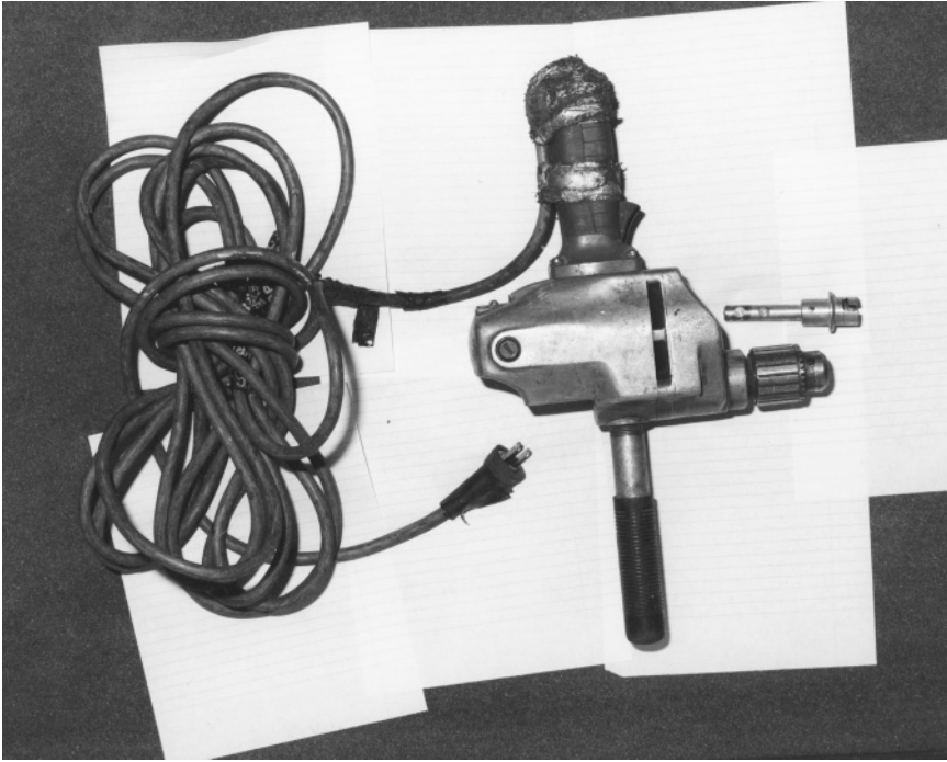
Figure 4.7 Heavy-duty drill with an adapter which allowed it to overload a sewer auger cable.
