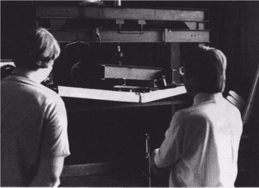
Figure 8.17 Full-scale laboratory load test of foam-filled sandwich panel.
