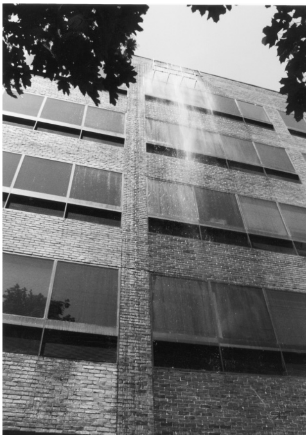
Figure 8.16 In-field water test on building cladding.
