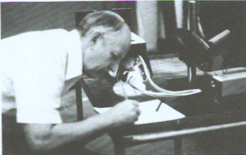
Figure 1.3 Analysis of results from the tests conducted using the apparatus shown in Figure 1.2. The analyst is studying the failure of the box-beam connection that supported the pedestrian walkways.
