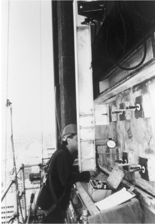
Figure 8.11 In-field pull-out tests on stone anchors.
