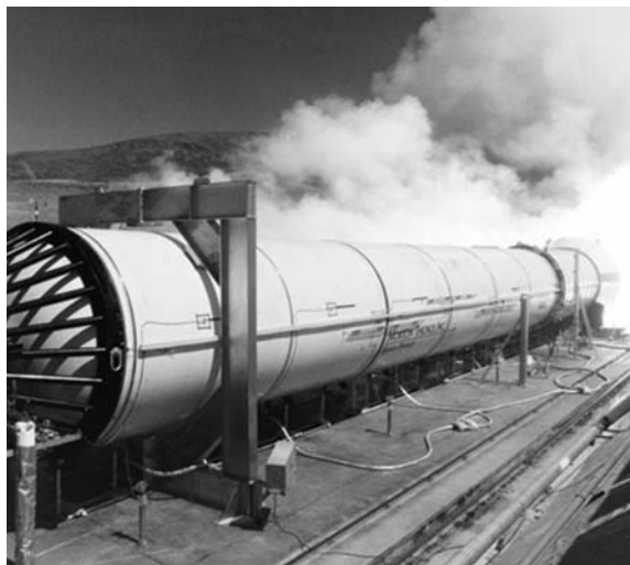
Morton-Thiokol tests a redesign of the solid rocket booster after the explosion of the space shuttle Challenger.
