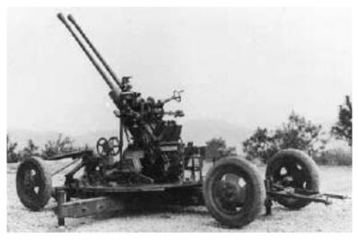
Crew 5 to 8 Length 5.94 m Width 1.90 m Height 2.08 m Weight 2,353 kg **Gun Caliber** 37 x 253mm FRAG-T, AP-T Ammuntion Type of Feed Clip (5 rds) Rate of fire 160 to 180 rds/min **Tactical AA range** 2,500/4,000 m Optical mechanical/radar Fire control
