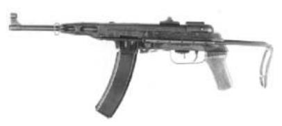
Caliber 7.62-mm **Effective Range** 100 m Cyclic Rate of Fire 900 rds/min
