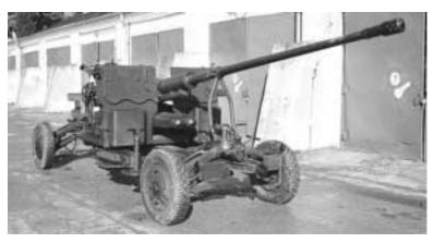
**Combat Weight** 4,773 kg Caliber 57 x 348-mm Rate of fire 105 to 120 rds/min
