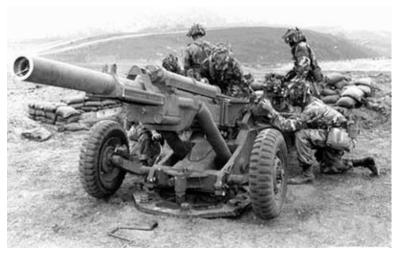
8 Crew Maximum Range 15,100 m Rate of Fire 10 rds/min **Combat Weight** 1,496 kg Length 5.18 m Width 1.96 m 1.594 m Height Prime Mover 6 x 6
