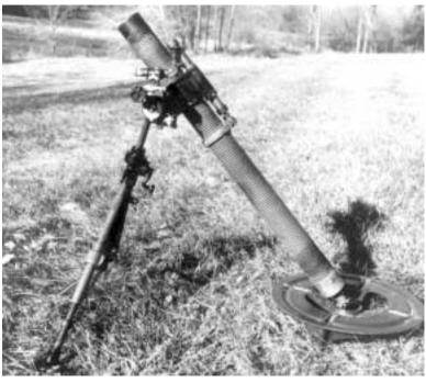
Crew Feed Length of Barrel Elevation 2 Muzzle loaded 1.295 m 800-1,500 mils
