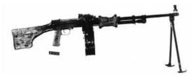
Caliber7.62 x 39-mmSystem of OperationGas, automatic
