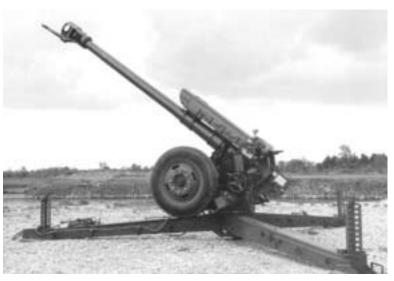
Crew 10 **Combat Weight** 3,210 kg Length 8.7 m Width 2.4 m 2.5 m Height Max Range 17,200 m Sustained Rate of Fire 2 rds/min **Prime Mover** Heavy 6 x 6 truck
