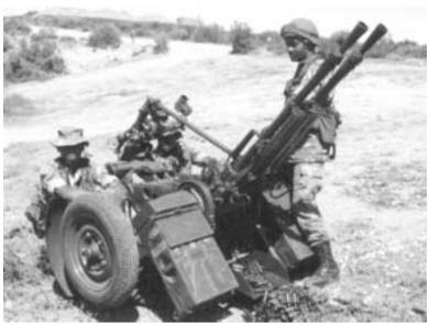
Crew5Maximum Range5,950 m m (horizontal) 3,700 m (vertical)Rate of Fire (Per Barrel)150 - 600 rds/minCombat Weight994 kg
