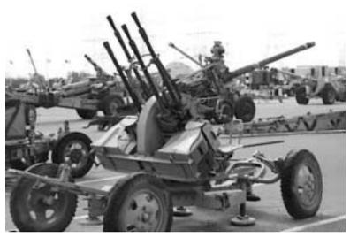
Crew5Maximum Range5,950 m (horizontal) 3,700 m (vertical)Rate of Fire (Per Barrel)550 - 600 rds/minCombat Weight1,810 kg
