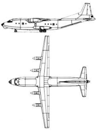
Type Wingspan Maximun Speed Maximum Range Payload Length Transport 38 m 419 kt 3,600 km 20,000 kg 33.1 m
