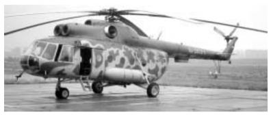
Crew4ArmamentAssorted Rockets and Gun PodsMaximum Speed160 ktsMaximum Range257 nmRotor Diameter21.29 m m
