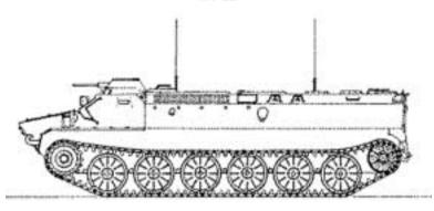
Crew/Passengers 2 + 11 Type Tracked Armament 1 x 7.62-mm PKT MG w/2,500 rds **Maximum Speed** 61.5 km/h Maximum Range 500 km **Fuel Capacity** 450 liters **Combat Weight** 11,900 kg Length 6.45 m Width 2.86 m 1.865 m Height Night Vision yes NBC yes Fording amphibious Gradient 60%
