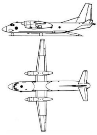
Type Wingspan Maximum Speed Maximum Range Payload Length transport 29.2 m 237 kt 1,100 km 5,500 kg 23.8 m
