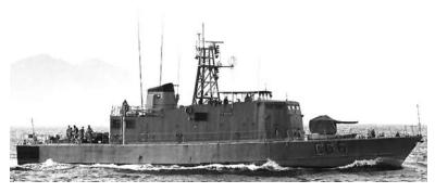
LOA x Max. Beam x Max. Draft40.6 x 6.7 x 1.6 mDisplacement, Full Load200 metric tonsComplement22 plus 9 spare berths
