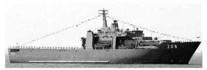
Type Complement LOA x Beam x Draft Displacement Military Lift Cruising Speed Helicopters Missiles Guns Radar Tank landing ship 65 141 x 21 x 5 m 8,500 t, full load 350 troops; 18 tanks; 20 vehicles; 4 LCVPs 15 kn 2x Super Puma 2 x Matra Simbad twin launchers for Mistral Otobreda 76-mm/62 Super Rapid Elta EL/M-2238 E/F-band air/surface search
