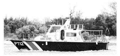
Type Complement LOA x Beam x Draft Displacement Cruising Speed Range Guns Radar Patrol craft 4 (plus 8 spare berths) 14.5 x 4.2 x 1.2 m 20 t, full load 30 kn 310 nmi 7.62-mm machinegun Furuno or Racal DECCA Bridgemaster I-band surface search PX 1 to PX 33 Patrol Craft
