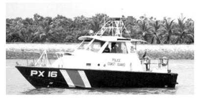
Type Complement LOA x Beam x Draft Displacement Cruising Speed Patrol 3 11 x 3.2 x 0.5 11 t, full load 30 kn
