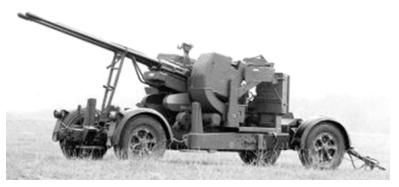
Crew Operation Maximum Range Rate of Fire Combat Weight Travel speed Prime Mover 3 Gas, automatic feed 4,000 m (vertical) 550 rounds/minute (per barrel) 6,300 kg Towed up to 60 km/h 5-ton (6x6) truck
