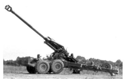
Crew 6 Caliber 155 mm x 39 caliber Maximum Range 30,000 m Rates of Fire Sustained 2 rounds/minute Maximum 6 rounds/minute 3 rounds in 15 seconds Burst **Travelling Weight** 12,800 kg Elevation -3 to +70 Traverse 60 degrees Traveling Length x Width x Height 9.16 x 2.8 2.29 m Gradient 45 degrees 0.76 m Fording Prime Mover 6 x 6 truck NOTE: The FH88 replaced the Soltam 155-mm M-71S.
