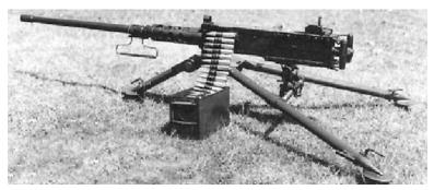
Effective Range Caliber System of Operation Overall Length Feed Device Weight (Loaded) 1,500 m 50 caliber (12.7 x 99-mm) Short recoil 1.651 m 100-round disintegrating-link belt 38 kg
