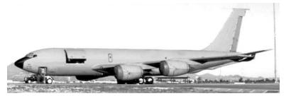
Mission Total Mission Time Cruising Speed Operating Weight, Empty Maximum Takeoff Weight Length x Wingspan x Height Mid-air refueling 5.5 hours 856 km/h 44.663 kg 134,715 kg 41.53 x 39.88 x 11.68 m
