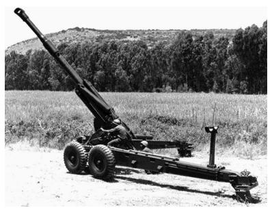
Crew8Maximum Range30,000 mRate of Fire5 rounds/minute (sustained 2 rounds/minute)Combat Weight9,200 kgLength x Width x Height7.5 x 2.58 x 2.12 mPrime Mover6 x 6 truckNOTE: The M-71S is the Israeli Soltam M-71 upgraded by Singapore
