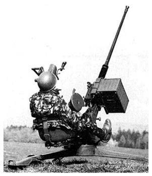
Crew Caliber System of Operation Effective Vertical Range Rate of Fire Feed Elevation Traverse Weight (no ammunition) Length x Width x Height (Firing) Towing Vehicle 3 (1 on gun) 20 mm Gas, auto, single (C01) or dual feed (C04) 1,500 to 2,000 m 1,050 rounds/minute (cyclic) 75-round box magazine (x1 for C01, x2 C04) -7 to +83 degrees 360 degrees 535 kg 3.87 x 1.7 x 1.45 m Light 4x4 truck
