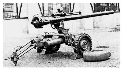
Caliber Maximum Range Rate of Fire Elevation Traverse Rifle Weight 105 mm 6,900 m (indirect fire) 5 rounds/minute -17 to +22 degrees 360 degrees 113.9 kg (combat order)
