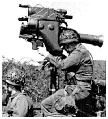
Range and Flight Endurance Night Vision Device Warhead Type Warhead Penetration Guidance/Command Link Attack Profile Launch Platforms 2,000 m in 12.5 seconds Thermal imaging Unitary shaped charge 1,000 mm of RHA SACLOS/Wire Direct line of sight Ground tripod, compact turret
