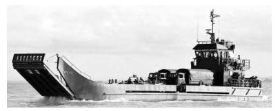
Type Complement LOA x Beam x Draft Displacement Cruising Speed Military Lift Mechanized landing craft 6 36.7 x 8.5 x 1.8 m 151,000 kg 10.7 kn 2 tanks, 450 troops, or 110 tons of cargo
