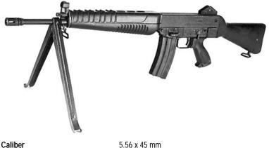
Caliber Fire Modes System of Operation Effective Range Cyclic Rate of Fire Feed Device Overall Length Weight (unloaded) 5.56 x 45 mm Automatic and semiautomatic Gas piston 400 m 600 to 800 rounds/minute 20- or 30-round box magazine 0.97 m 3.7 kg
