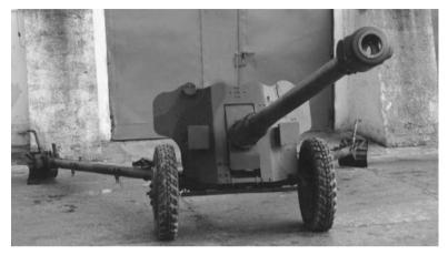
Crew Caliber Max Range Rate of fire Combat Weight Length Width Ammunition Towing Vehicle 8 85-mm 15,650 m 15-20 rds/min 1,703 kg 8.34 m 1.78 m AP-T, AT-T, and HVAP-T
