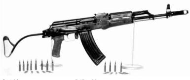
Cartridge Rate of Fire System of Operation Overall Length Magazine Capacity Weight (Empty) 5.45- x 39-mm Cyclic; 600 rds/min Gas, selective fire Standard and folding models, butt extended, 940 mm 30- or 40-round detachable box magazine 3.41 kg
