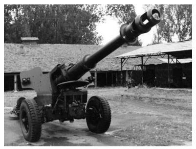
Caliber Max Range Rate of fire Combat Weight Length Width Ammunition 152-mm 24,000 m 2-4 rds/min 7,500 kg 7.105 m 2.53 m OF-540 HEI, OF 559 HEI, BR540 AP HEAT, Leaflet
