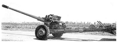
Crew8Max RangeOF-412 HE-FRAG projectile 20,700 m<br/>APC-T projectile 4,000 m<br/>HEAT projectile 2,200Conversion time/travel to firing mode60 secondsCombat Weight3,200 kgLength9.37 mWidth2.24 mNOTE: Ammunition fired by M1977 is identical to that used in the T-54/55 MBTs.
