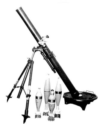
Maximum Range Rate of Fire Combat Weight Length of Barrel 4,500 m (5,700 m HE extended-range) 20 rds/min 47 kg 1.44 m
