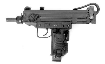
Cartridge Rate of Fire Caliber System of Operation Overall Length Magazine Capacity Weight (Loaded) 9- x 19-mm Parabellum or 9- x 18-mm Makarov Cyclic; 700 rds/min 9-mm Conventional blowback Butt extended 710 mm (Parabellum); 625 (Makarov) 25-round box magazine (32-rd for Makarov) 2.75 kg
