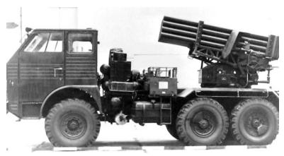
Crew Capacity Reload time Max Effective Range Vehicle Speed Vehicle Range Vehicle Combat Weight Vehicle Length Vehicle Length Vehicle Width NBC System Night Vision 1-5 40 barrels, 122-mm 15 minutes 20,380 m 80 km/h (road); 25 km/h (cross-country) 1,000 km 17,650 kg 7.39 m 2.51 m Yes Yes
