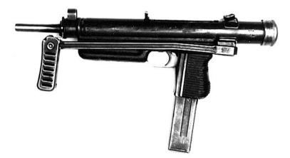
Cartridge Rate of Fire Caliber System of Operation Overall Length Magazine Capacity Weight (Loaded) 9- x 19-mm Parabellum Cyclic; 650 rds/min 7.62 x 25-mm (pistol type P) Blowback, selective fire 686 mm 32-round box magazine 3.41 kg
