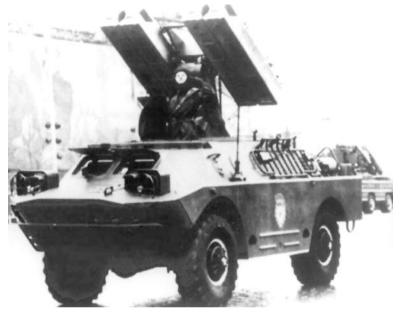
Type Guidance Maximum Range Maximum Altitude Launch Weight Length Low altitude surface-to-air missile system Passive IR homing seeker 4,200 m 3,000 m 30 - 30.5 kg 1.803 m
