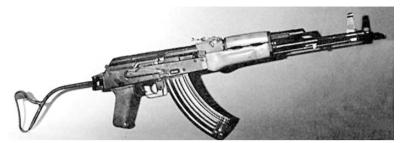
Maximum Effective Range Caliber System of Operation Rate of Fire Magazine Capacity Overall Length Weight (Empty) 500 m 7.62- x 39-mm Gas, selective-fire Cyclic, 600 rds/min 30-rd, detachable box magazine 879 mm 3.15 kg
