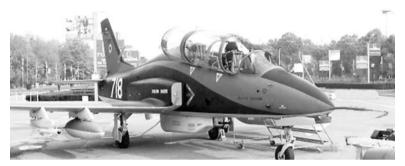
Type Armament Maximum Speed Max Range Length Height Max Take-off Weight Advanced jet trainer/light attack jet Assorted rockets, missiles, and bombs 865 km/h) 1,100 km (with internal fuel) 11.01 m 3.90 m 5,480 kg
