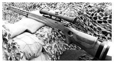
Maximum Effective Range Caliber System of Operation Overall Length Magazine Capacity Weight (Loaded) 800 m 7.62-mm Bolt action, repeater 1.15 m 5-round, detachable box magazine 4.9 kg
