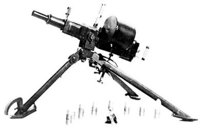
Operation Maximum Range Rate of Fire Feed Weight (with Full Drum) Length Width Height Blowback 1,300 m Cyclic, 300-400 rds/min 10-round drum magazine 43 kg 1.46 m 775 mm 600 m
