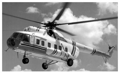
Type Crew/Passengers Armament Max Speed Range Payload Length Width Height Twin-turbine multipurpose helicopter 2/28-32 Assorted machineguns, bombs and missiles 260 km/h 425 km (with 24 passengers) 4,000 kg 25.24 m 2.50 m 5.65 m
