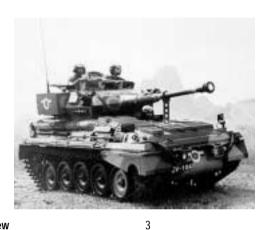
Crew Armament Main 1 x 90-mm gun Coaxial 1 x 7.62-mm MG Smoke 2 x 4 **Night Vision** Yes **NBC Capable** Yes Maximum Road Range 756 km Maximum Speed 72.5 km/h **Fuel Capacity** 391 liters Fording 1.06 m Gradient 60% Vertical Obstacle 0.5 m **Combat Weight** 8,723 kg 2.1 m Height 5.28 m Length Width 2.26 m
