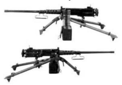
Maximum Effective Range Caliber System of Operation Overall Length Feed Device Weight (Loaded) 1,500 m .50 caliber Browning (12.7-mm x 99) Short recoil 1.651 m 100-rd disintegrating link belt 38 kg
