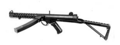
Maximum Effective Range Caliber System of Operation Overall Length Feed Device Weight (Loaded) 200 m 9-mm x 19 Parabellum Blowback, selective fire 28 in stock extended, 19 in stock folded 34-rd curved box magazine 6 lbs
