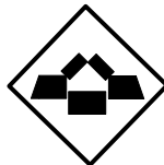
Opening or swing bridge
