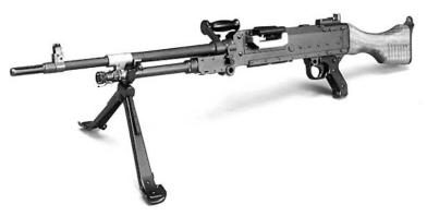
Maximum Effective Range Caliber System of Operation Feed Device Weight (Loaded) Overall Length 1,500 m 7.62- x 51-mm NATO Gas, automatic Belt 13.92 kg (with butt stock and bipod)
