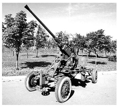
Crew5 to 8Gun Caliber37 mm x 253Ammunition TypesFRAG-T, AP-TFeed5-rd clip
