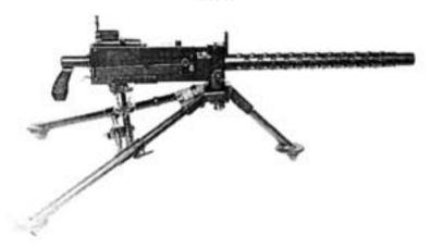
Maximum Effective Range Caliber System of Operation Feed 1000 m .30 caliber or 7.62-mm Automatic Belt fed
