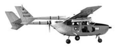
Crew1ArmamentAssorted rockets, missiles, and gun podsMaximum Speed172 ktsMaximum Range545 nmWingspan11.63 m
