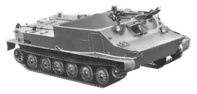
Crew/Passengers Type Armament Maximum Speed Maximum Range Night Vision NBC Fording Gradient Vertical Obstacle Trench 2 + 14 tracked 1 x 7.62-mm MG w/1,250 rds 45 km/h 240 km yes yes amphibious 60% 1.1 m 2.8 m M113
