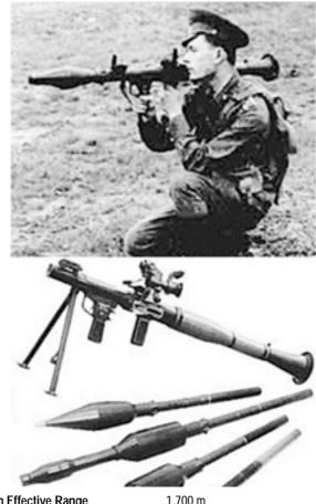
Maximum Effective Range Caliber Overall Length 1,700 m 30-mm 1.1 m
