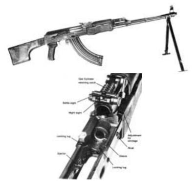
Maximum Effective Range Caliber System of Operation Overall Length Magazine Capacity 800 m 7.62 x 39-mm gas, selective fire 48.2 in. 40-rd, staggered row detachable box magazine or 75-rd drum magazine. Can also use 30-rd AK magazine 1.13 kg (40-rd box) 2.1 kg (75-rd drum)
