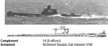
Maximum Speed (kts) Maximum Range, Miles Displacement (t) LOA/Beam/Draft m(f) 54 (8 officers) McDonnel Douglas Sub Harpoon SSM 8 x 21 in. tubes (6 bow and 2 stern) w/14 Allient Mk37F Mod 2 28 mines in lieu of torpedoes 16 (surfaced) 13 (submerged) 9,000 @ 9 kts (surfaced) 1,475 tons (surfaced) 1,830 tons (submerged) 76.6 x 6.7 x 4.9 (251.3 x 22.0 x 16.1)
