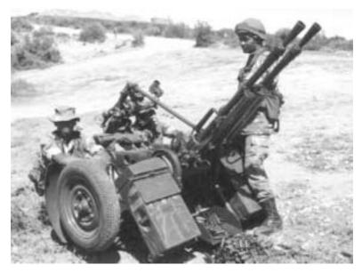
Crew Maximum Range Rate of Fire (Per Barrel) Combat Weight Length Width Height 4 8,000 m (horizontal) 5,000 m (vertical) 150 - 600 rds/min 1,810 kg 4.53 m 1.72 m 2.13 m
