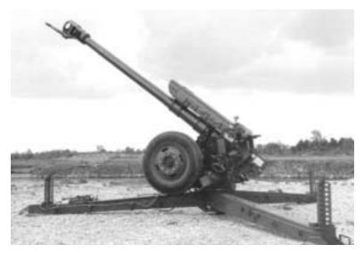
Crew Maximum Range Rate of Fire Combat Weight Length Width Height Prime Mover 7 15,400 m (conventional) 21,900 m (RAP) 7 rds/min 3,210 kg 5.4 m 1.95 m 1.66 m 6 x 6 truck
